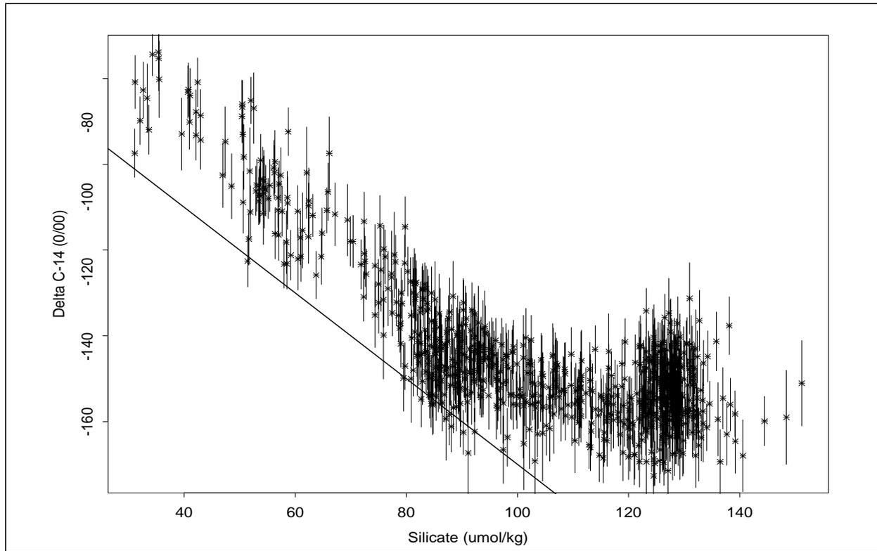
**Figure 3:**  $\Delta^{14}\text{C}$  as a function of silicate for S4I AMS samples. The straight line shows the relationship proposed by Broecker, *et al.*, 1995 ( $\Delta^{14}\text{C} = -70 - \text{Si}$  with radiocarbon in ‰ and silicate in  $\mu\text{mol/kg}$ ). Two-sigma error bars are given for the  $\Delta^{14}\text{C}$  measurements.
