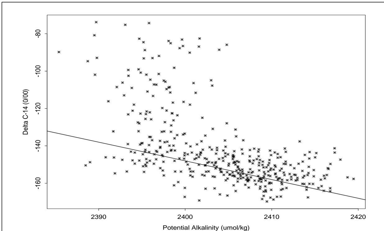
**Figure 4:** Based on the new method devised by S. Rubin, the samples which plot above the line and have potential alkalinity values less than about 2400  $\mu\text{mole/kg}$  are contaminated with bomb-produced  $^{14}\text{C}$ .
