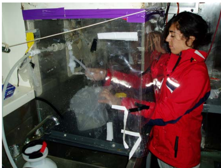
Figure 3: Natalie Cohen filling a cubitainer for our Fe/vitamin amendment grow-out experiment at Station Papa using the IOS trace metal clean sampling pump system.
