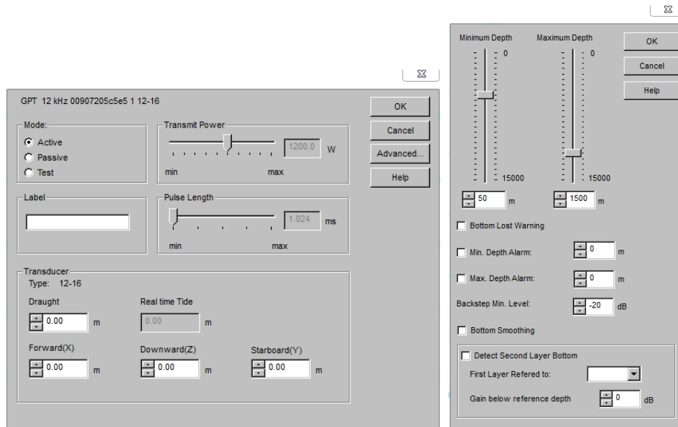
Figure 8: Echosounder settings for 1000 m of water. (Left) This menu is accessed by right clicking on the “12 kHz” square in the upper left corner of the screen. (Right) This menu is accessed by right clicking on the top bar behind the depth reading.
