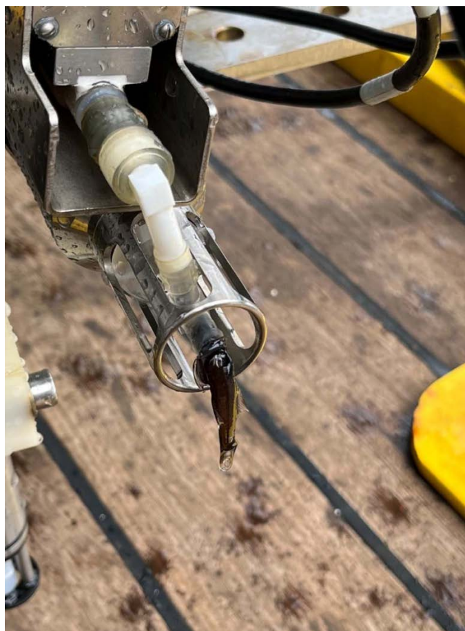
Figure 6.1 Fish blocking primary SBE 3P inlet.
