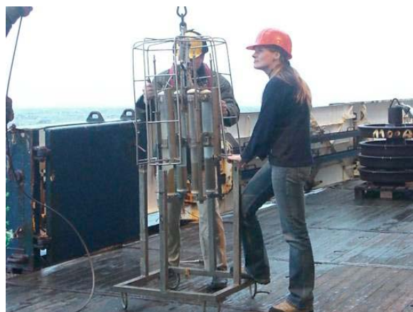
Fig. 3.28: Minicorer deployment during ANT-XXIV/3
