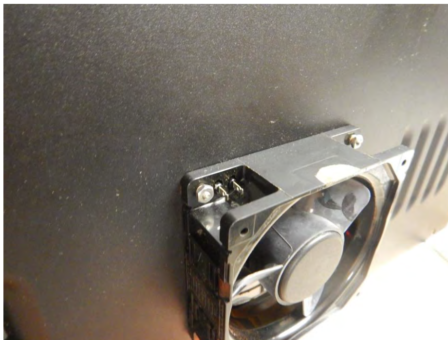
Figure 11:- Autosol S/N 65753 Disconnected Exhaust Fan
