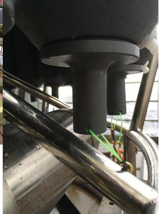
Figure 17:- 20 L CTD bottle clearing stainless steel frame
