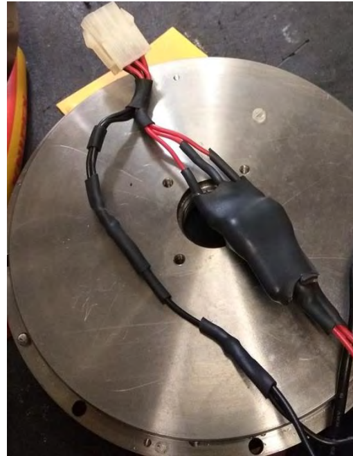
Figure 21:- Chelsea Battery Pack S/N 182042 Replacement charging components
