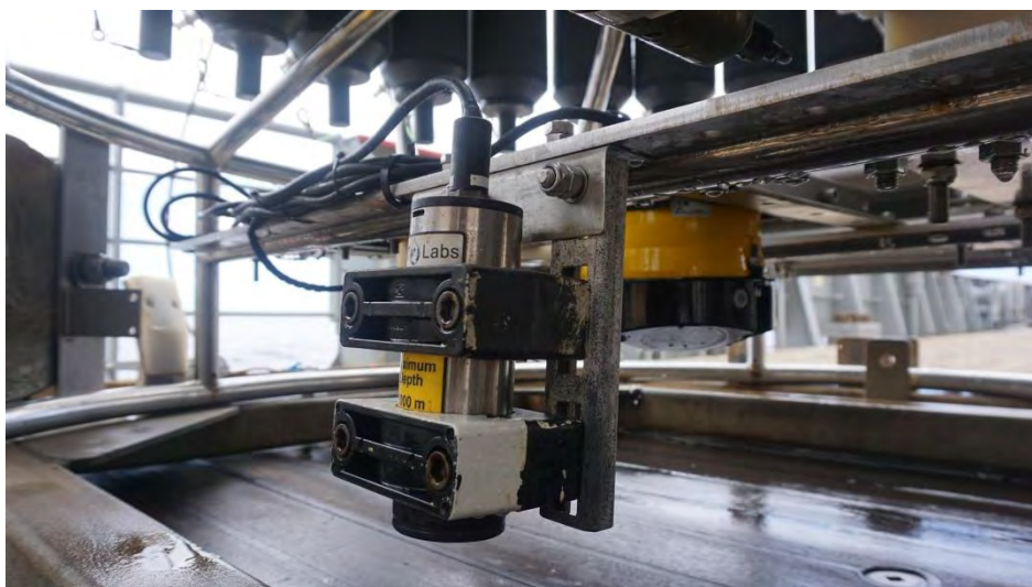
Figure 18:- Seabird Eco-FLBB installation
