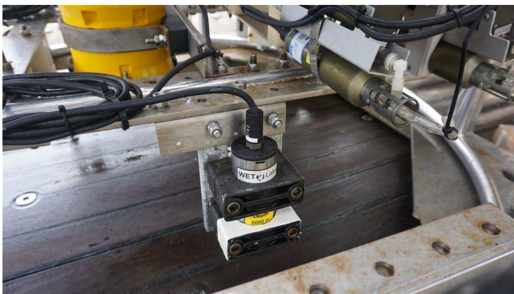
Figure 19:- Seabird Eco-FLBB installation
