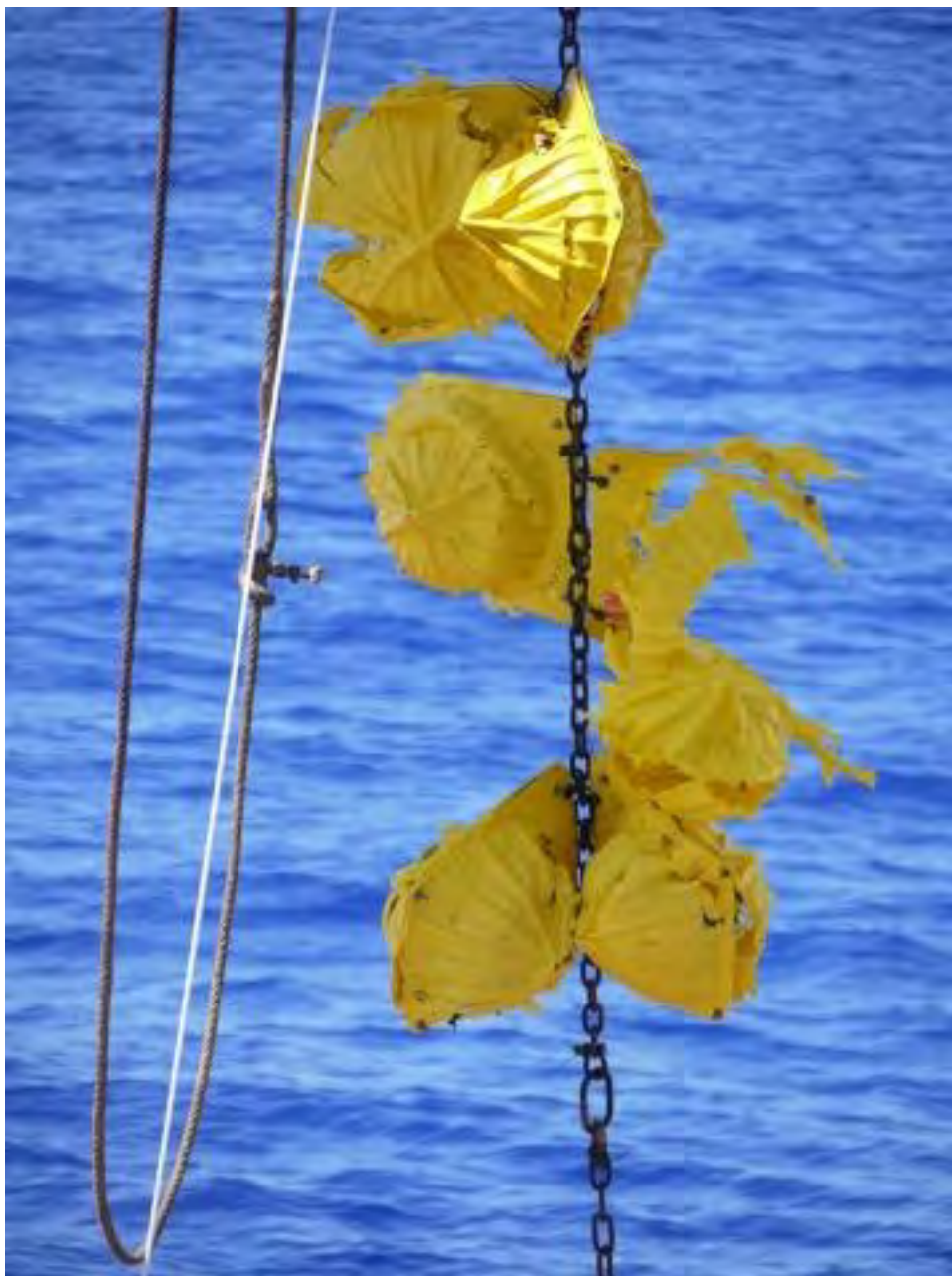
Figure 4: Imploded buoyancy spheres.
