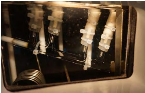
Figure 6:- Autosal S/N 65833 Cell Tubing Fault
