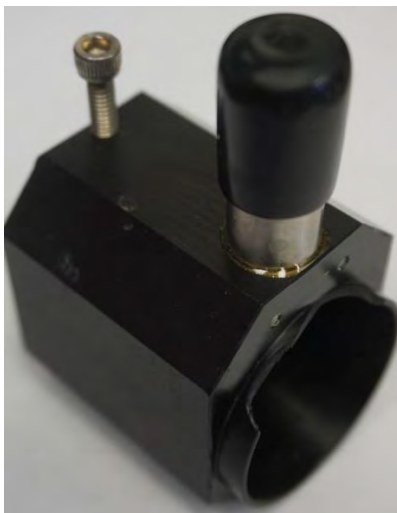
Figure 14:- Transmissometer bracket damaged end
