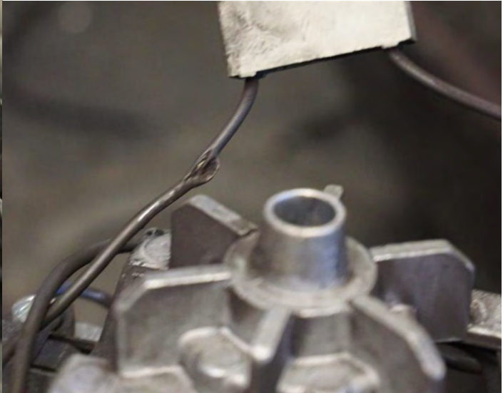
Figure 24:- UEA damaged capacitor wire
