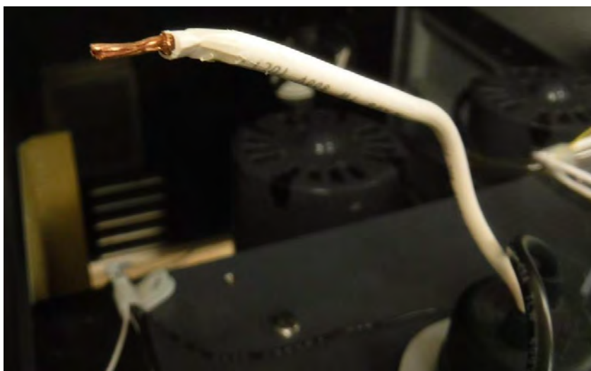
Figure 9:- Autosal S/N 65833 Broken heating lamp wire
