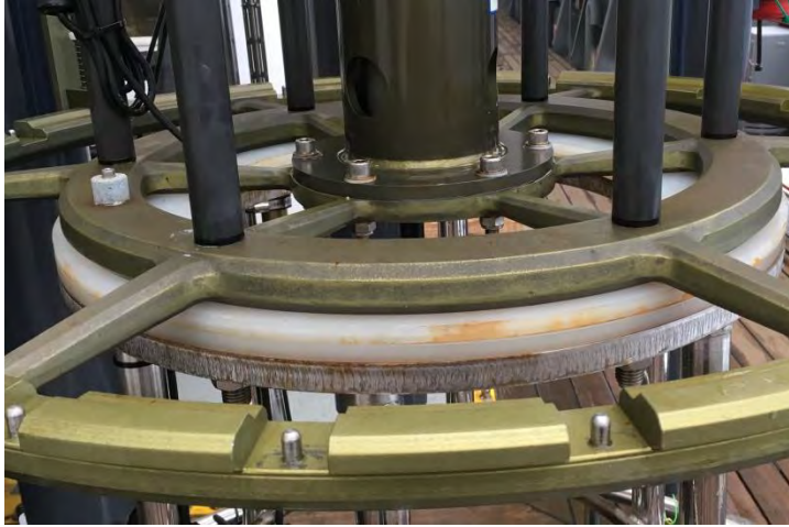
Figure 16:- Installation of additional CTD isolation washer
