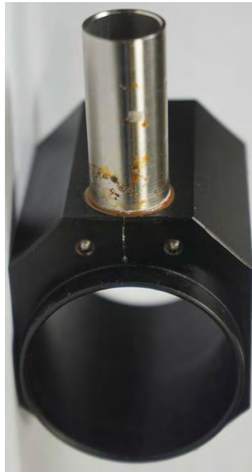
Figure 13:- Transmissometer end bracket hairline crack
