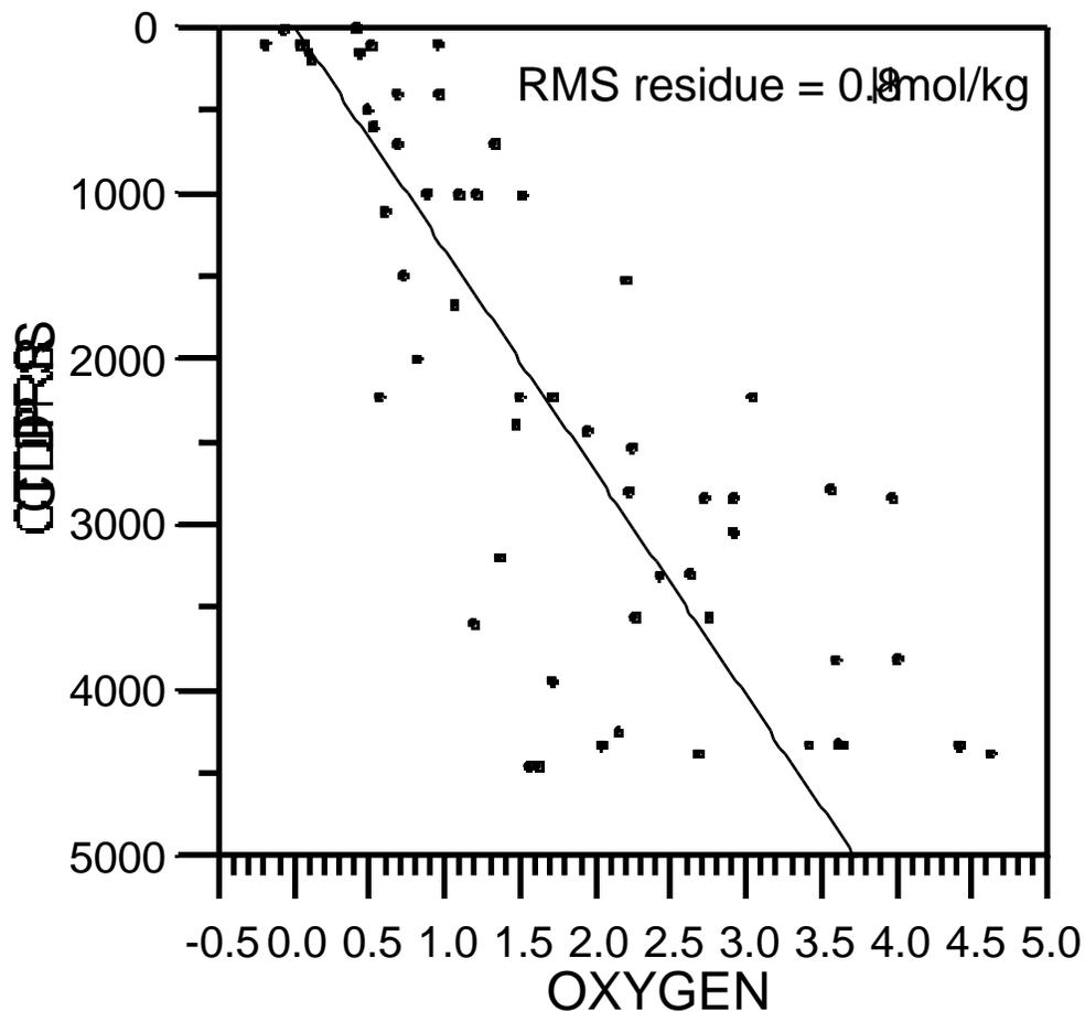
Figure 20. Difference of the oxygen concentration from water sampled with the NOEX sampler fitted with the silicon rubber ball lids water sampled with NOEX samplers with PETP lids. Plotted versus the sample pressure. The line gives the linear regression.
