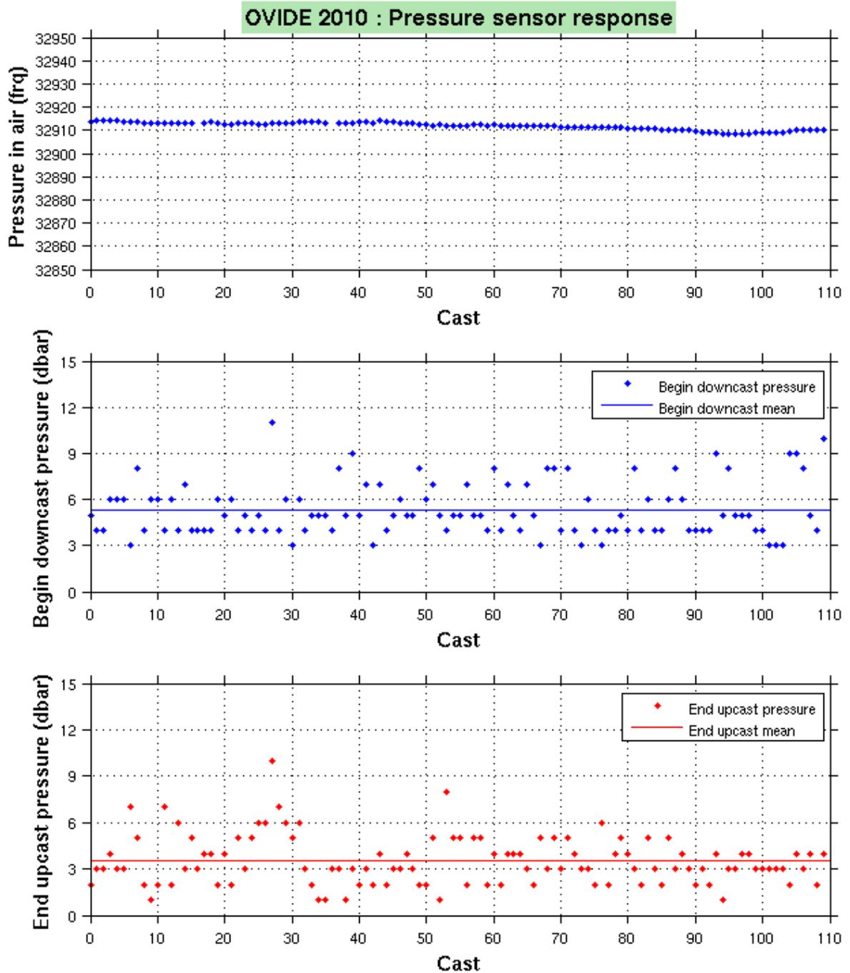
**Figure 9 :** Monitoring of the pressure sensor readings :
