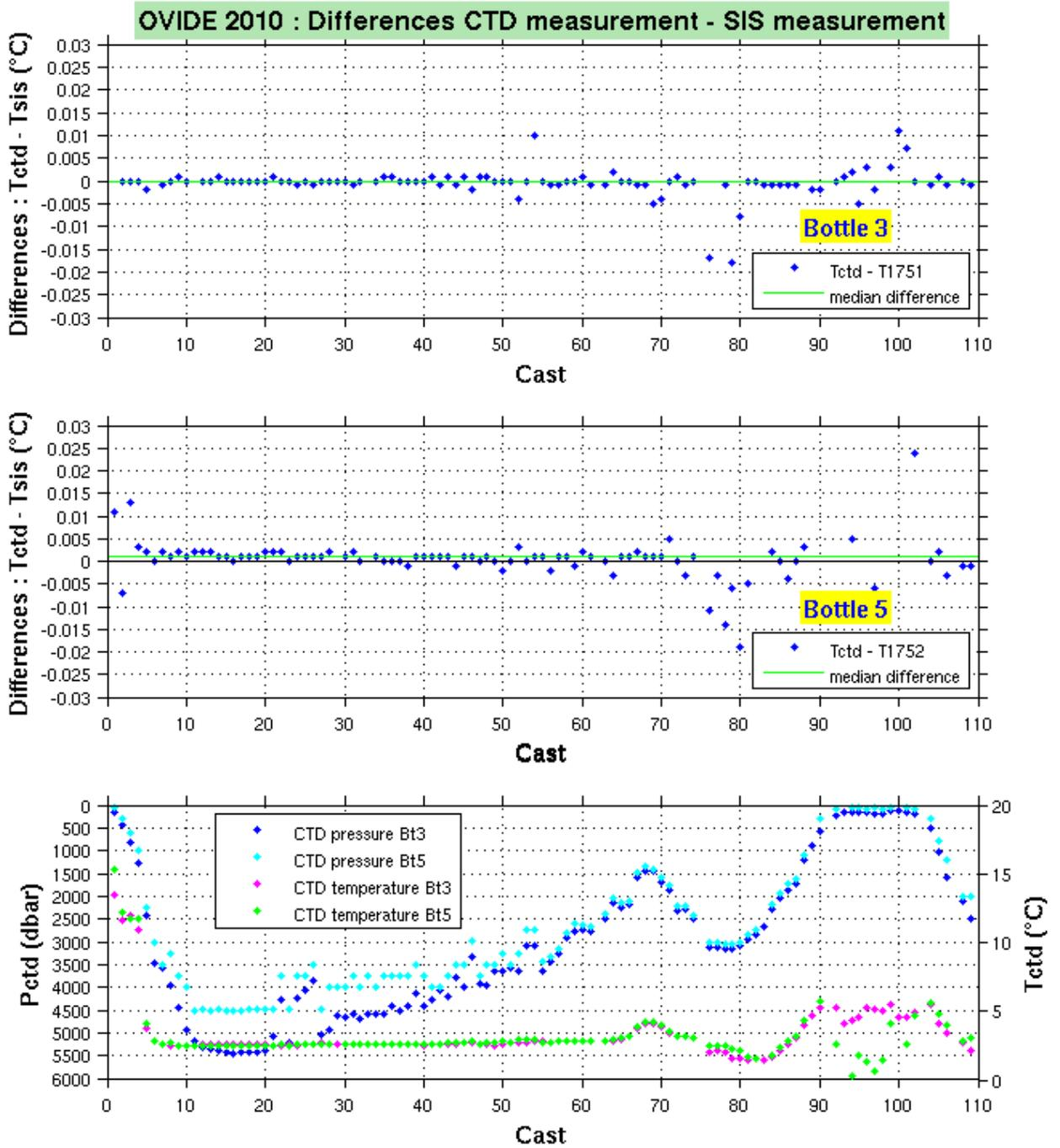
**Figure 12 :** Differences obtained, at each cast, between the SIS thermometer (1751 and 1752) readings and the temperature indicated by the Seabird probe. The bottom graph specifies the pressure and temperature values at the time of closure of bottles 3 and 5.
