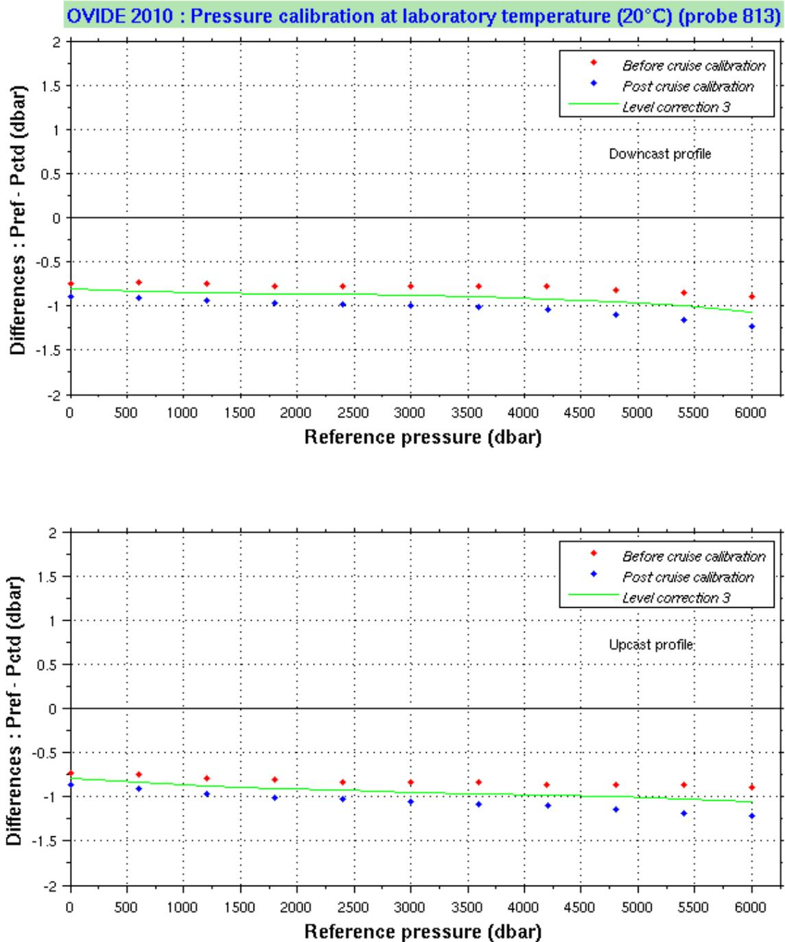
**Figure 7 :** Distribution of the mean differences, every 600 dbar, between the reference pressure and the pressure indicated by the Seabird sensor during pre-and post-cruise calibrations at laboratory temperature (20°C) :
