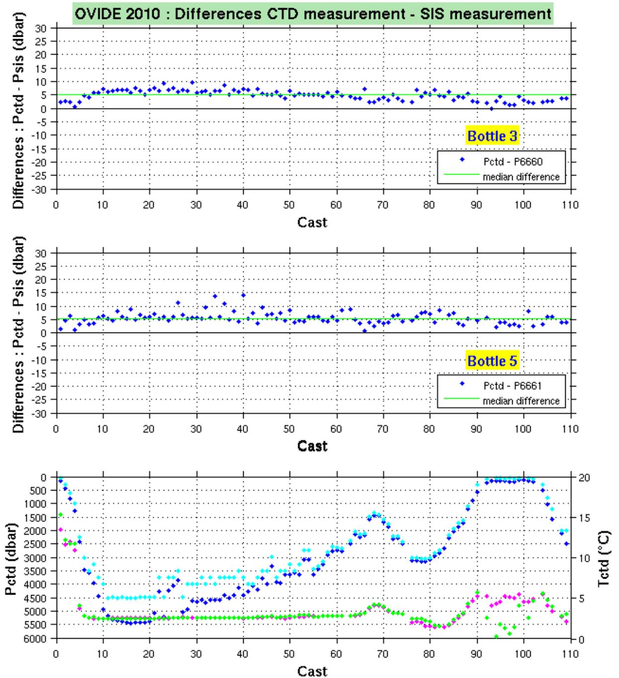
**Figure 10 :** Monitoring of the differences between the SIS pressure meters and the CTD pressure sensor. The bottom graph specifies the pressure and temperature values upon closure of bottles 3 and 5.
