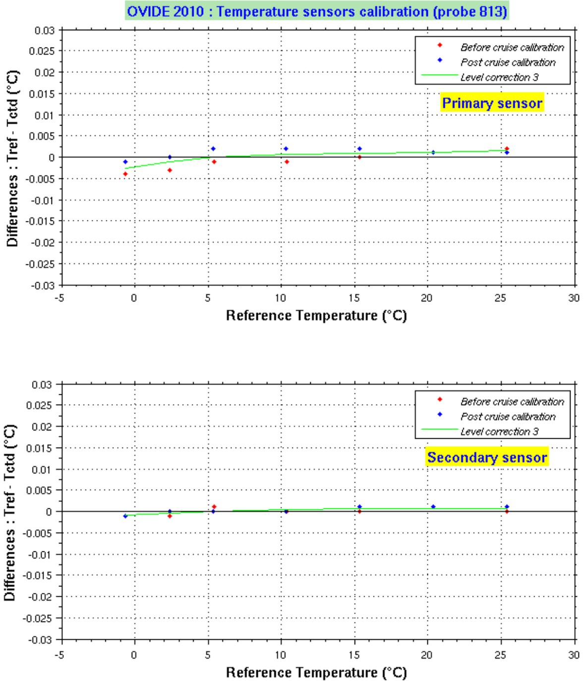
**Figure 11 :** Differences between the reference temperature and the temperature measured by the SBE3+ sensor (primary and secondary) during pre-and post-cruise calibrations. The optimal correction (degree 3) is shown as a solid line.
