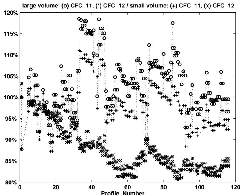
Figure 2: Temporal evolution of the ECD-efficiency during the cruise for the 0.5 mL volume (small) and the 2 mL volume (large).
