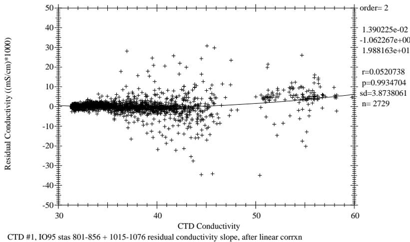
**Figure 8.3.2** CTD #1 residual non-linear conductivity slope (WOCE95 stations 801-856 + 1015-1076).
