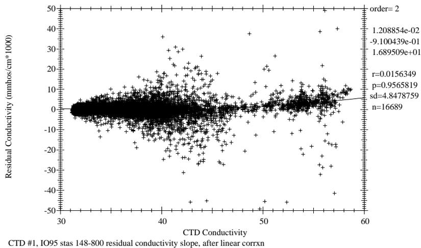
Figure 8.3.2 CTD #1 residual non-linear conductivity slope (WOCE95 stations 148 through 800).
