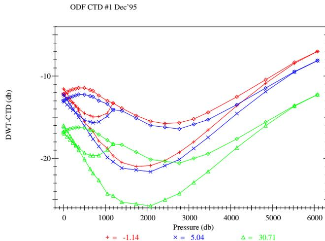
**Figure 7.1** Pressure calibration for ODF CTD #1, December 1995.
