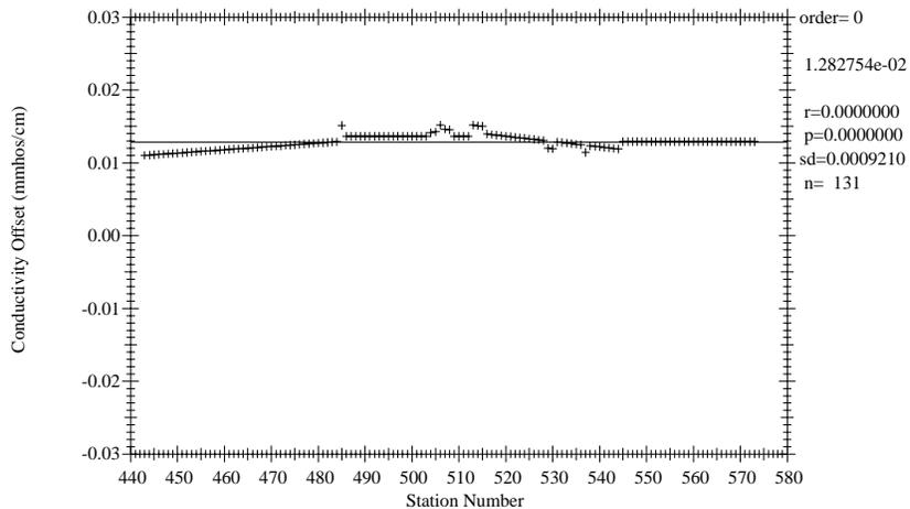
**Figure 8.3.4** I3 CTD #1 conductivity offsets by station number.
