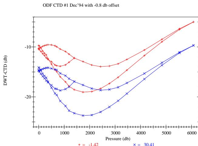
**Figure 8.1.0** I3 Pressure correction for ODF CTD #1: December 1994 calibration offset by  $-0.8$  db.
