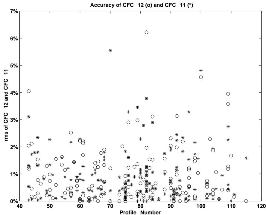
Figure 1: Accuracy of CFC-11 (\*) and CFC-12 (o); replicate samples plotted vs profile number.
