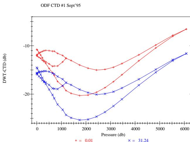
Figure 7.1 Pressure calibration for ODF CTD #1, September 1995.
