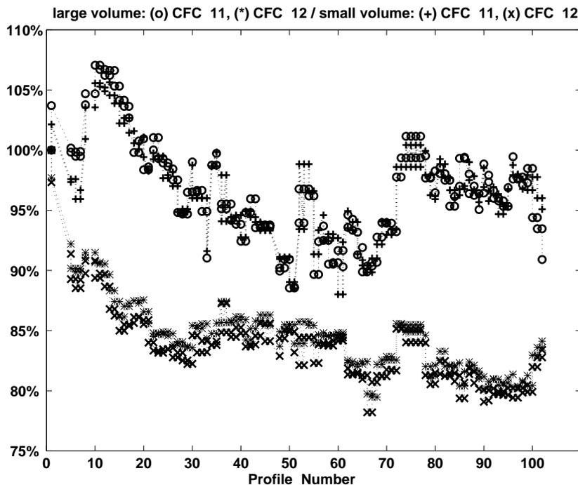
Figure 2: The temporal evolution of the ECD-efficiency during the cruise for the 0.5 ml volume (small) and the 2 ml volume (large).
