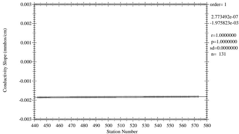
**Figure 8.3.3** I3 CTD #1 conductivity slope corrections by station number.
