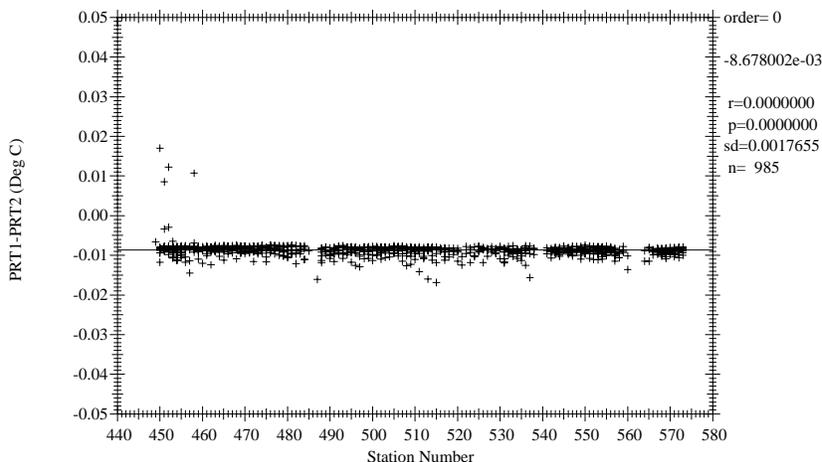
Figure 8.2.0 I3 Shipboard comparison of CTD #1 primary/secondary PRT temperatures, pressure > 1000 db.
