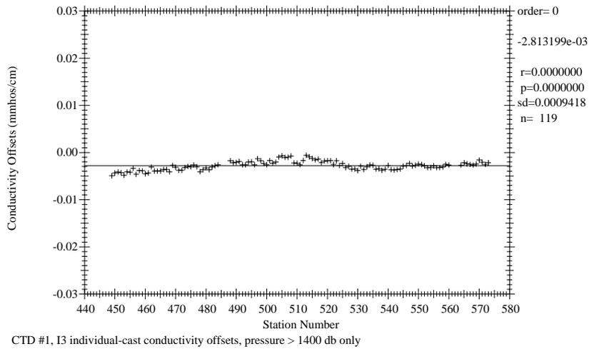
Figure 8.3.1 I3 CTD #1 preliminary conductivity offsets by station number.
