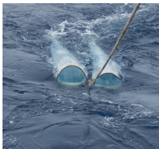
Figure 22: Horizontal towing of bongo net for surface zooplankton collection
