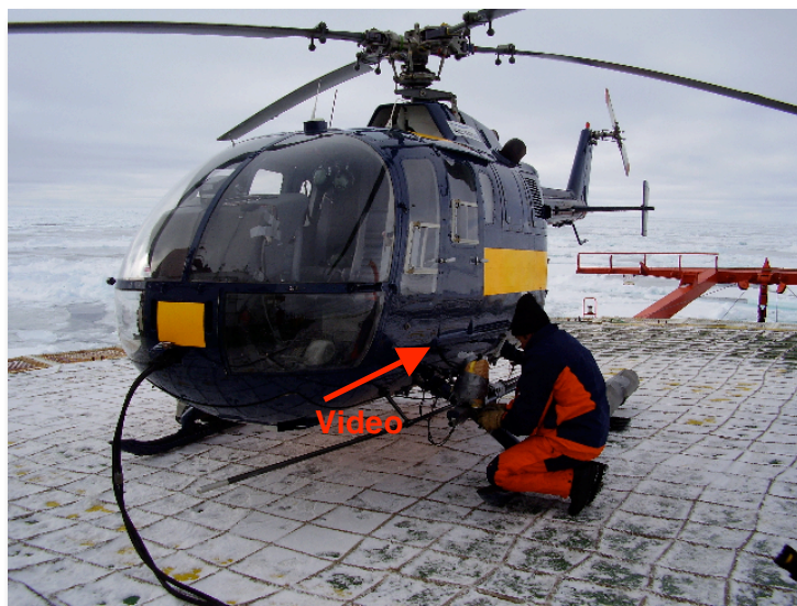
Fig. 4.30: Mounting a video camera on the helicopter
