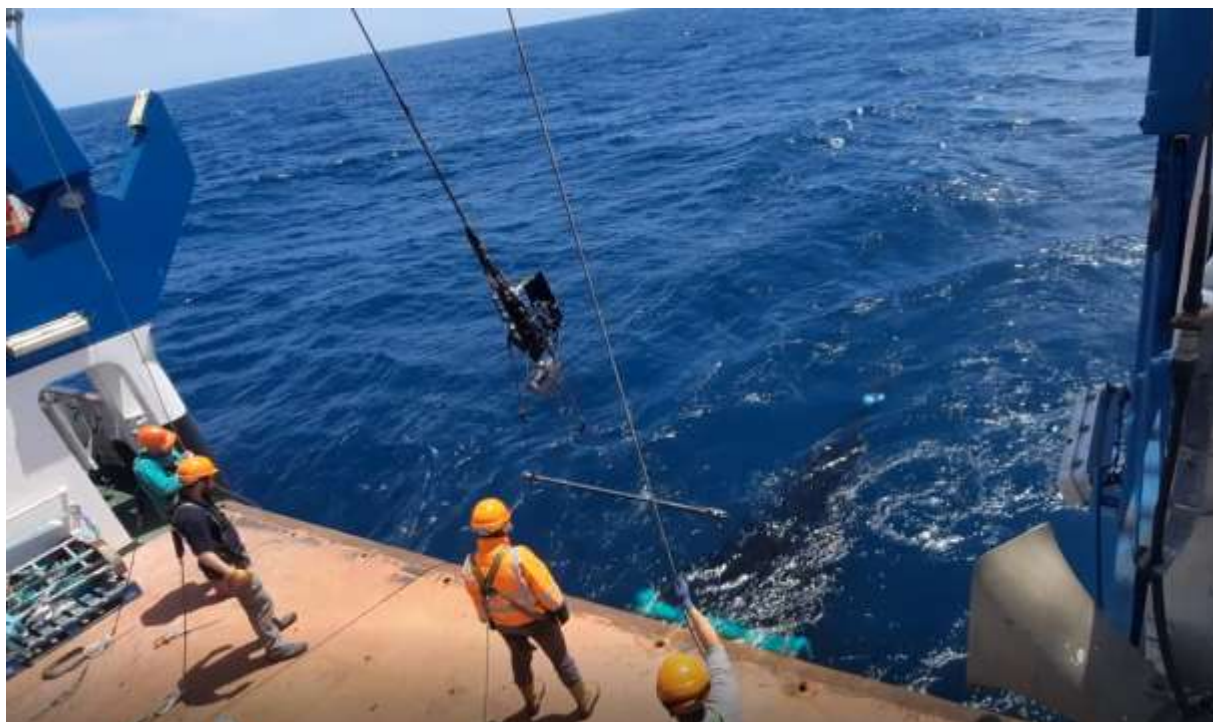
Figure 22. Recovery of RMT 8 net. Auxiliary wires yet to be connected to the weight bridles.
