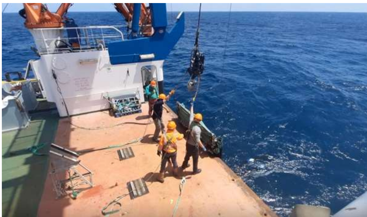
Figure 23. Recovery of RMT8 net. Auxiliary wires connected and weight bar in the process of being hauled on deck by auxiliary winches in tandem with the trawl winch.
