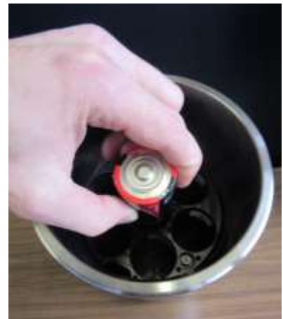
Figure 10. Installing batteries into a battery container.
