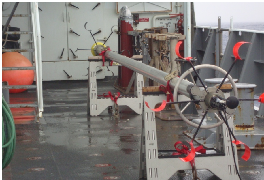
Fig. 6.2.1. A Shearmeter ready for launch.
