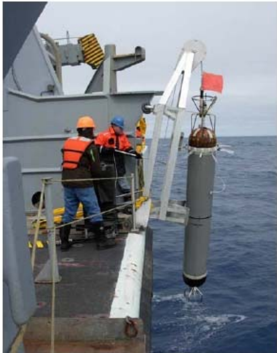
Fig. 3.2.4. Attaching tag lines to HRP for recovery, guiding HRP aft, lifting back aboard, and returning it to the hangar for data offload.
