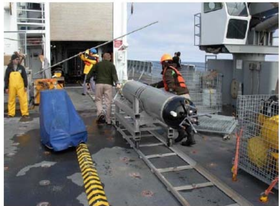
Fig. 3.2.4. Attaching tag lines to HRP for recovery, guiding HRP aft, lifting back aboard, and returning it to the hangar for data offload.
