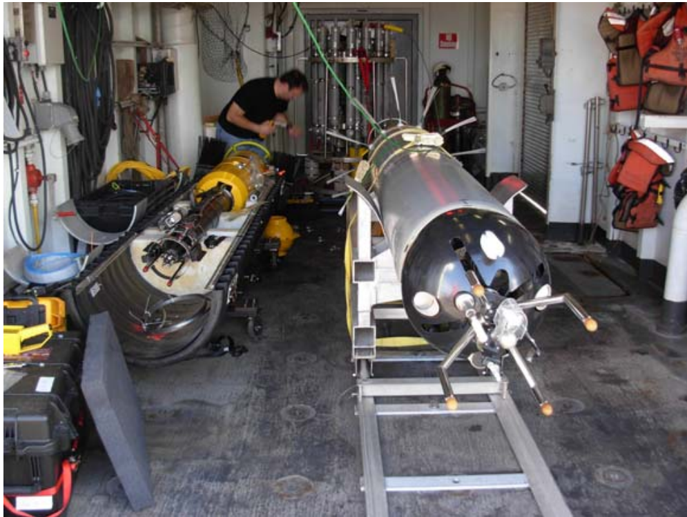
Fig. 3.2.1. The HRP-II (right) mounted in the deployment carriage inside the R/V Thompson hangar and the DMP (left) in its storage cradle.
