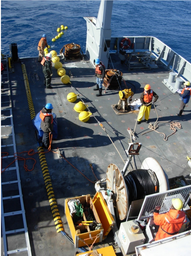
Fig. 4.2.1. Flotation spheres being eased off the deck and into the water.
