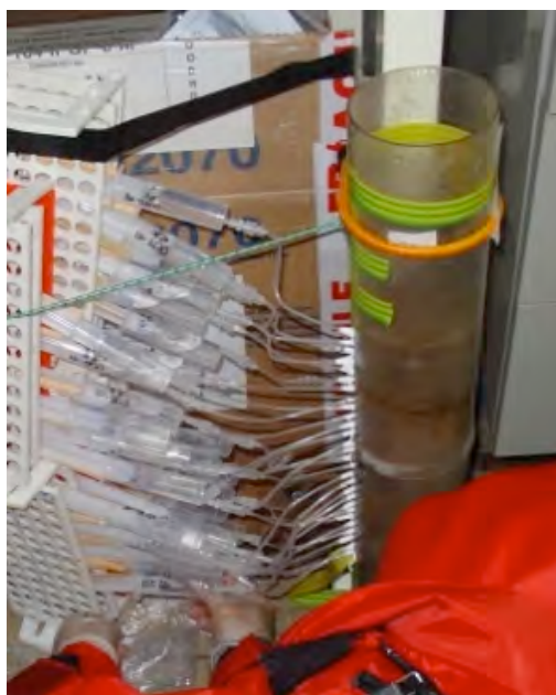
Figure 54 – In situ filtration with Rhizon® (porous probes, 0.2 μm)
