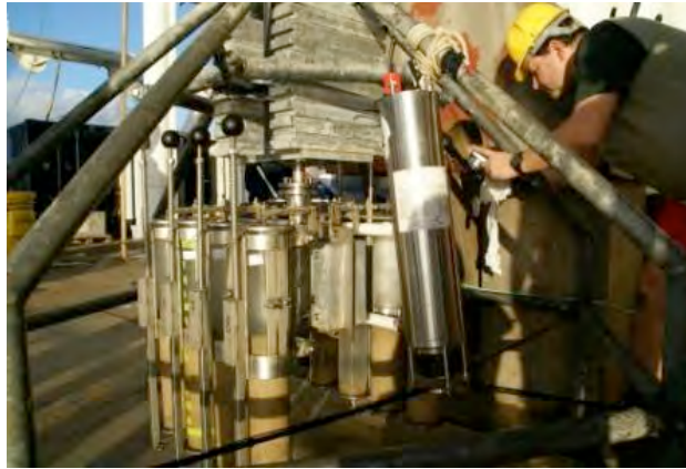
Figure 53 – Oktopus Gmbh multiple corer (head version MUC 8/100) equipped with 8 transparent polycarbonate cylinders deployed during the BONUS-GOODHOPE cruise
