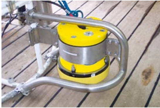
Figure 3.3: Detail of the LADCP frame mount.
