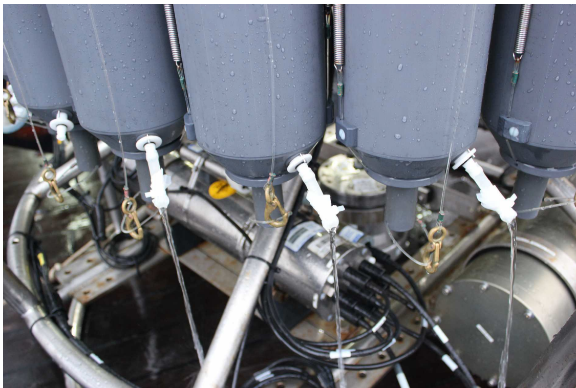
Figure 16.3: Rubber pipe with 80 \mu m mesh gauze screen fitted to the niskin bottle spigot, allowing for water filtration directly from the CTD to analyse microplastics in deep sea water.
