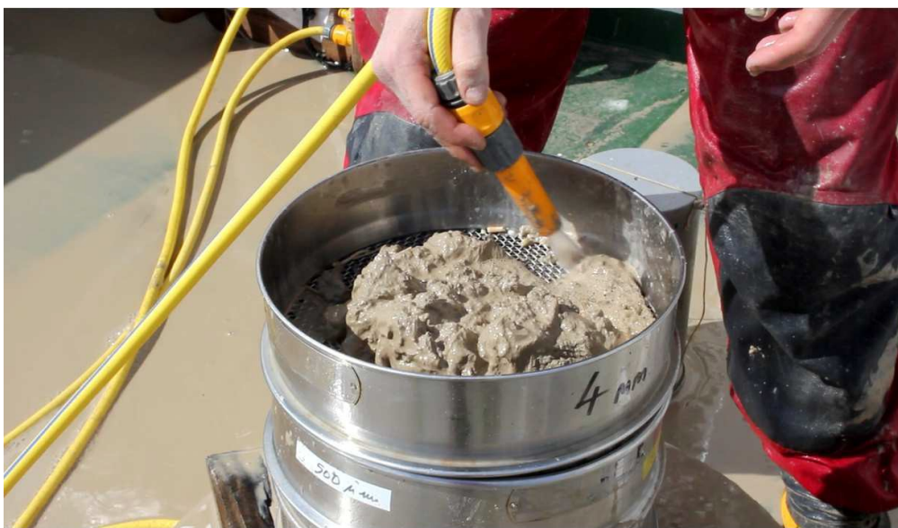
Figure 15.2: Stacked sieves
