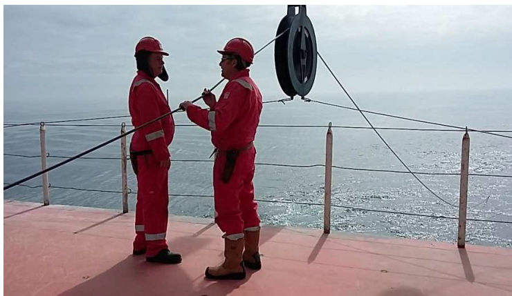
Figure 17.5: Hydrophone deployment
