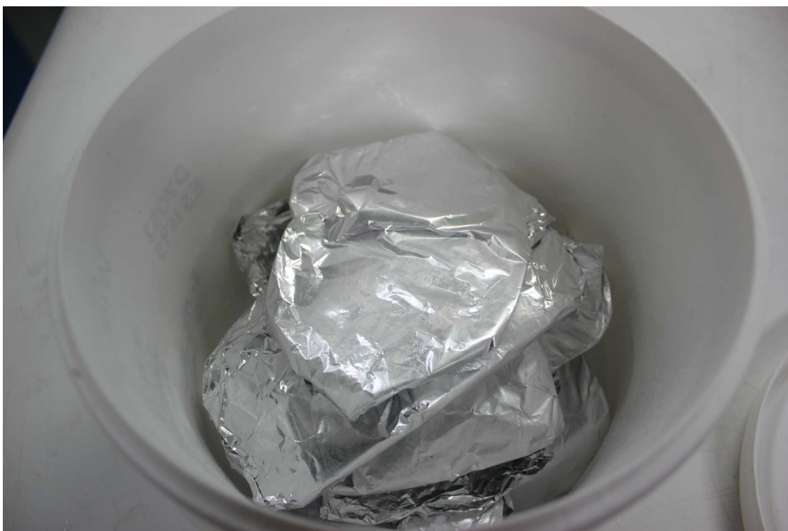
Figure 16.2: Invertebrate specimens individually wrapped in aluminium foil in clean sealable container
