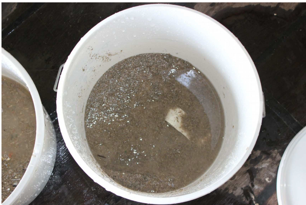
Figure 15.4: Sample collected on 0.42 mm sieve.
