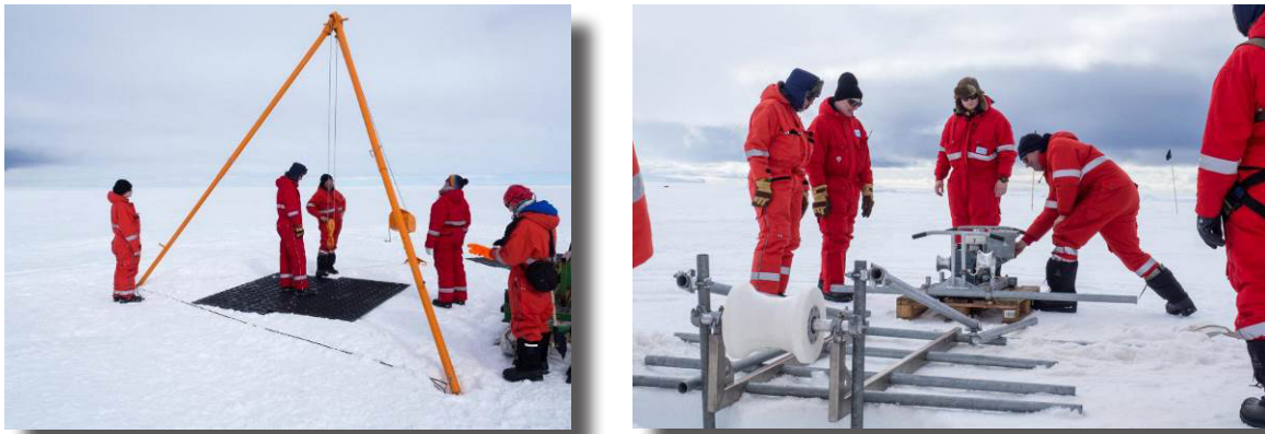
Fig. 3.1.1.9: Left: The tripod (test set-up, ultimately to be placed over the hole for lifting heavy instruments). The area covered by black plates (2 x 2 m) indicating the approximate size of the hole. Right: The rope-guidance at the edge of the hole for the recovery of the mooring rope. Pulling out the rope is supported by the portable capstan (behind the rope-guidance).
