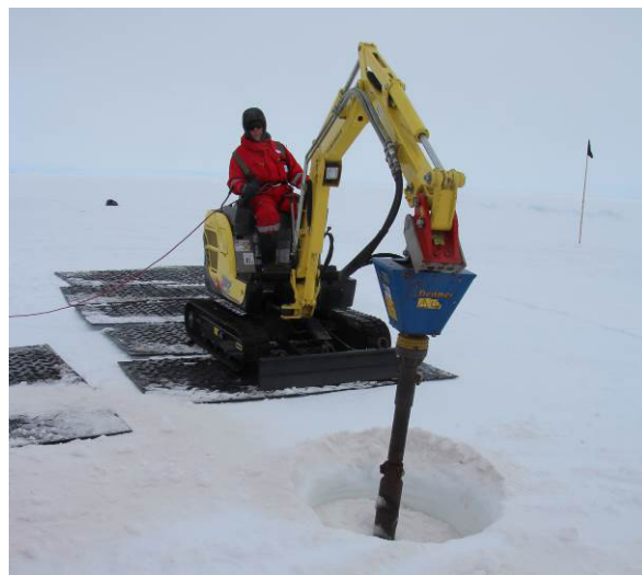
Fig. 3.1.1.8: Drilling a 90 cm diameter hole. Larger holes need to be created by overlapping several holes.
