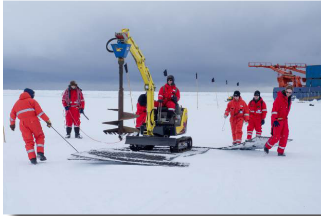
Fig. 3.1.1.7: The earthmover drives on plates to the drill site. The plates are necessary if the ice floes are covered with high and soft snow.
