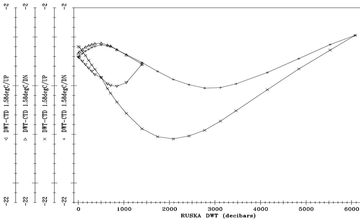
Figure 1a: CTD #1 Pre-cruise Cold Pressure Calibration
