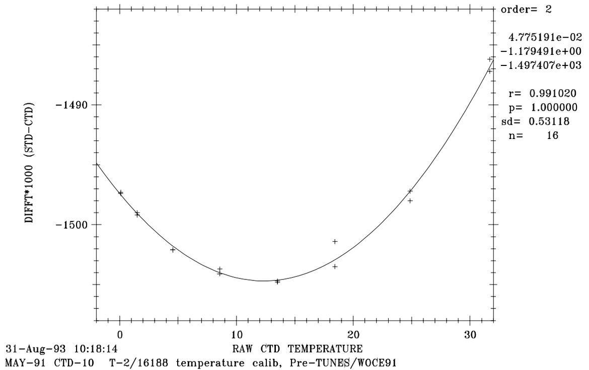
Figure 6b: CTD #10 Pre-cruise PRT-2 Temperature Calibration
