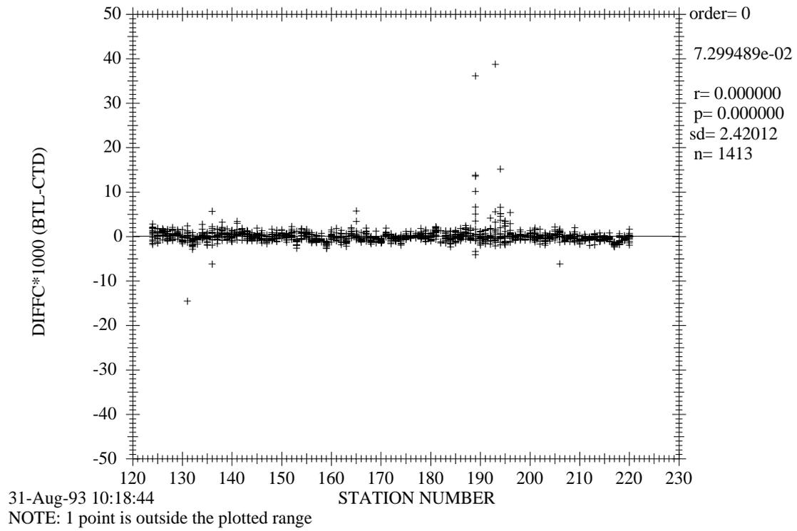
Figure 10b: TUNES-2 Residual Conductivity Bottle-CTD Differences - Prs>1500dbar
