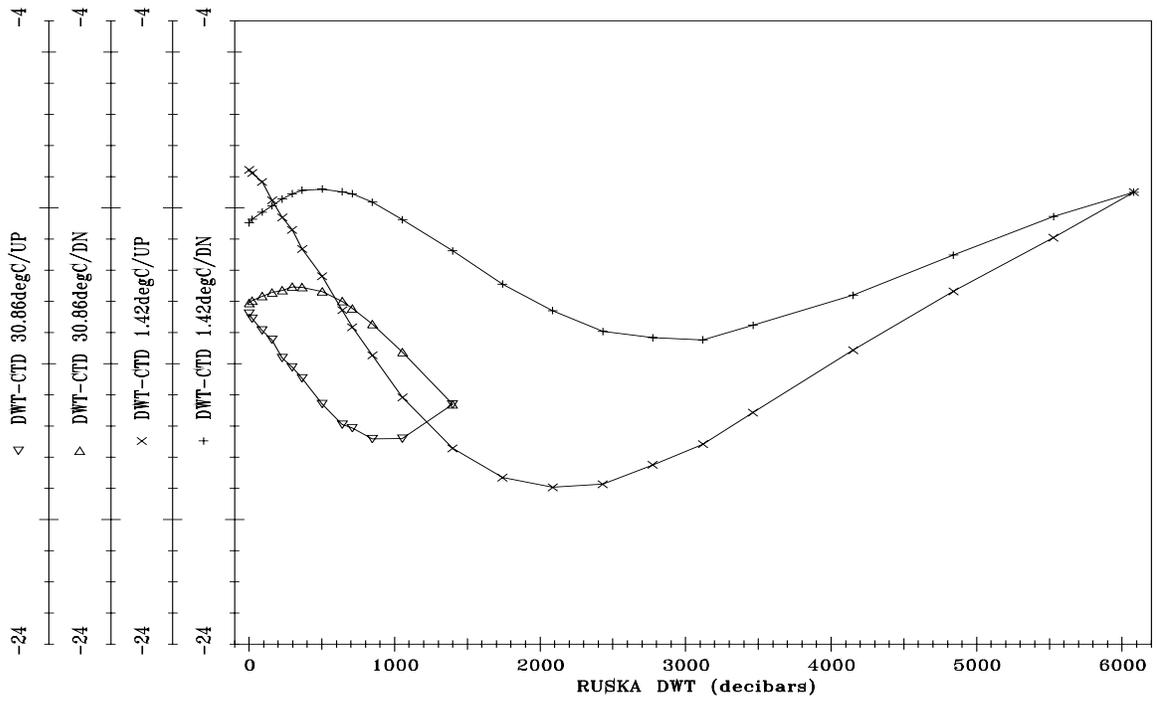
Figure 1c: CTD #1 Post-cruise Pressure Calibration
