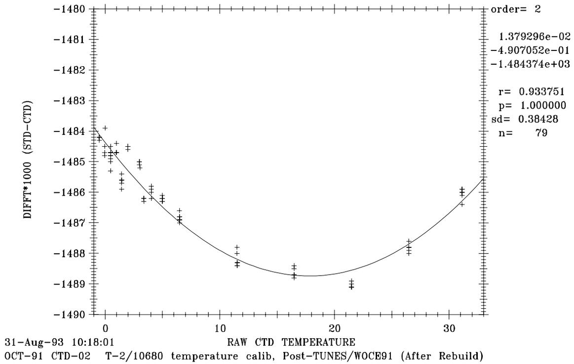
Figure 5d: CTD #2 Post-cruise PRT-2 Temperature Calibration
