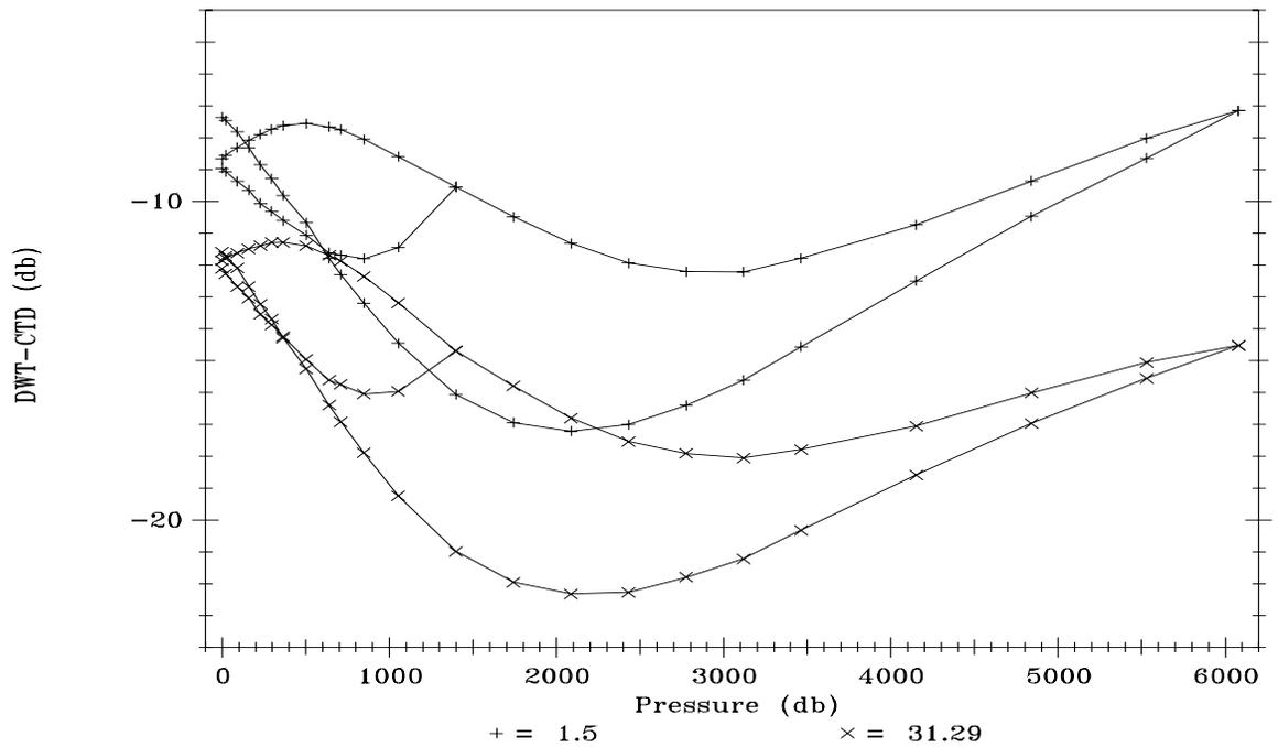
Figure 1d: CTD #1 Averaged Pre-/Post-cruise Pressure Calibration
