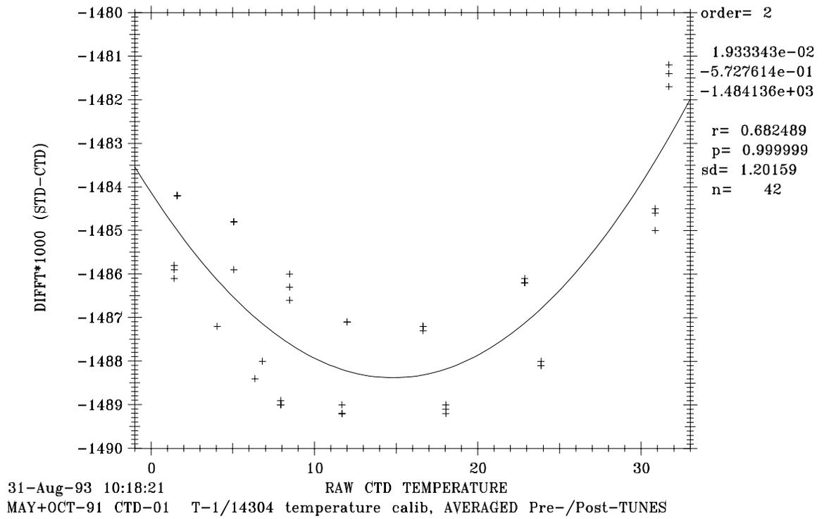
Figure 4c: CTD #1 Averaged Pre-/Post-cruise PRT-1 Temperature Calibration
