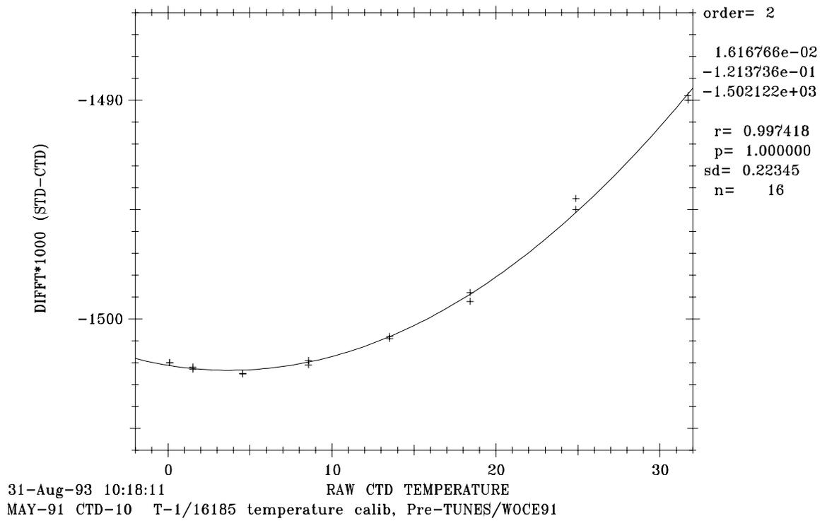
Figure 6a: CTD #10 Pre-cruise PRT-1 Temperature Calibration
