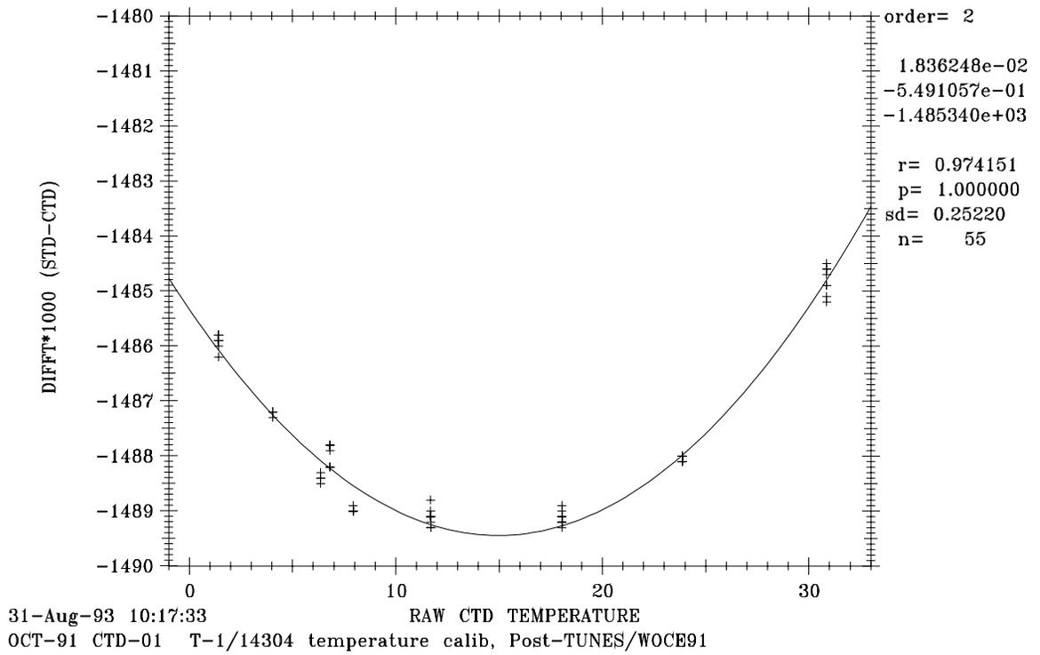
Figure 4b: CTD #1 Post-cruise PRT-1 Temperature Calibration
