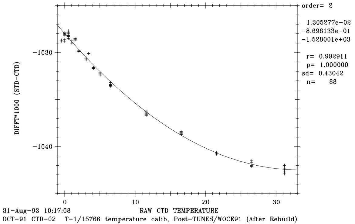
Figure 5b: CTD #2 Post-cruise PRT-1 Temperature Calibration
