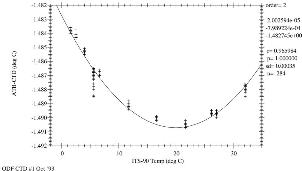
Figure 1.5.3 Temperature calibration for ODF CTD #1, October 1993.
