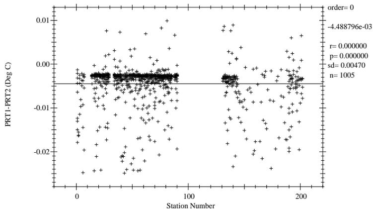
Figure 1.6.0 Comparison between the primary and secondary PRT channels.
