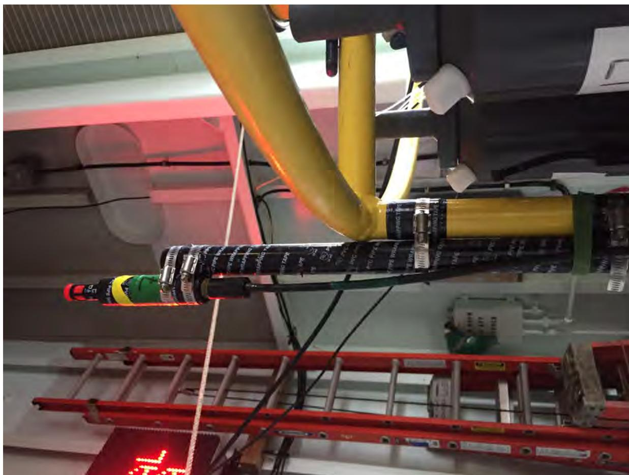
Fig. 1: Upward-looking chipod sensor attached to the rosette
