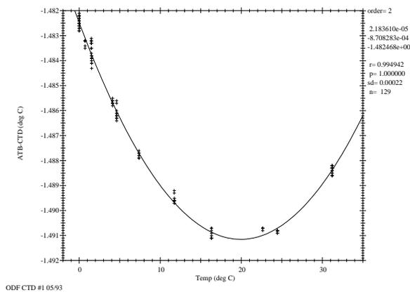
Figure 1.5.3 Temperature calibration for ODF CTD #1, May 1993.
