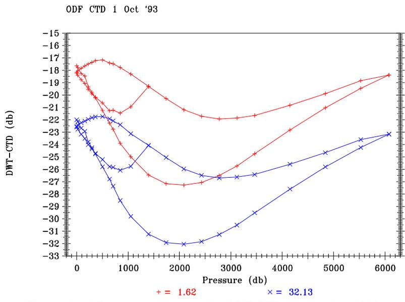
Figure 1.5.1 Pressure calibration for ODF CTD #1, October 1993.
