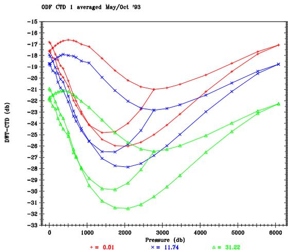
Figure 1.6.1 Pressure calibration for ODF CTD #1, averaged May/Oct 1993.
