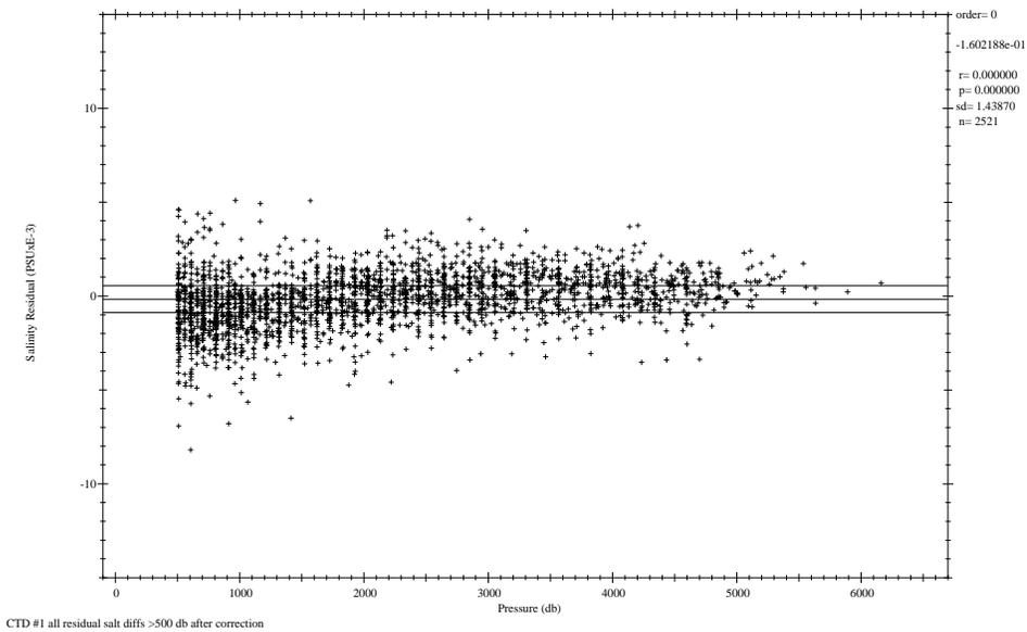
**Figure 1.6.3** Salinity residual differences vs pressure (after correction).
