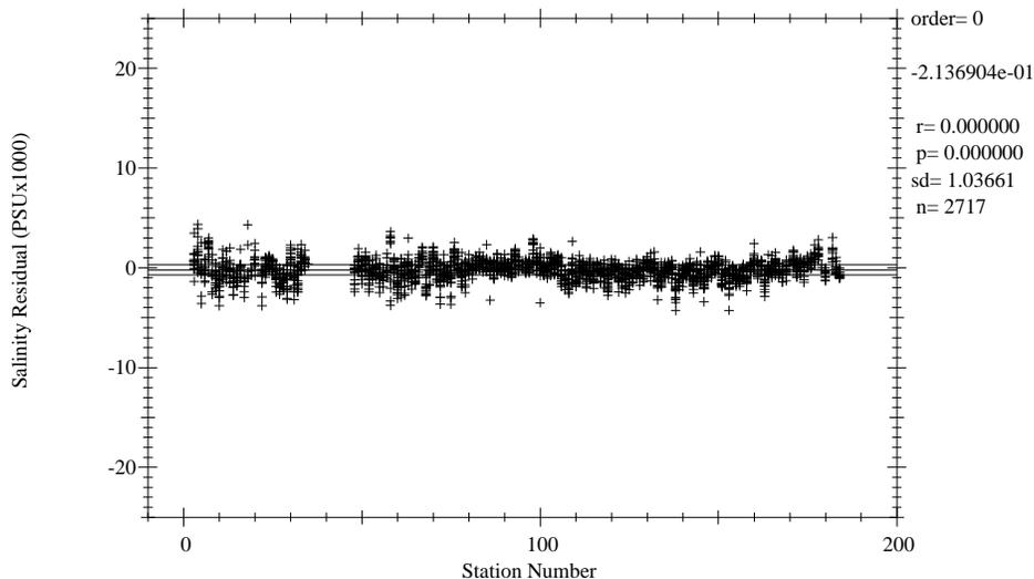
**Figure 1.6.5** Deep salinity residual differences vs station # (after correction).
