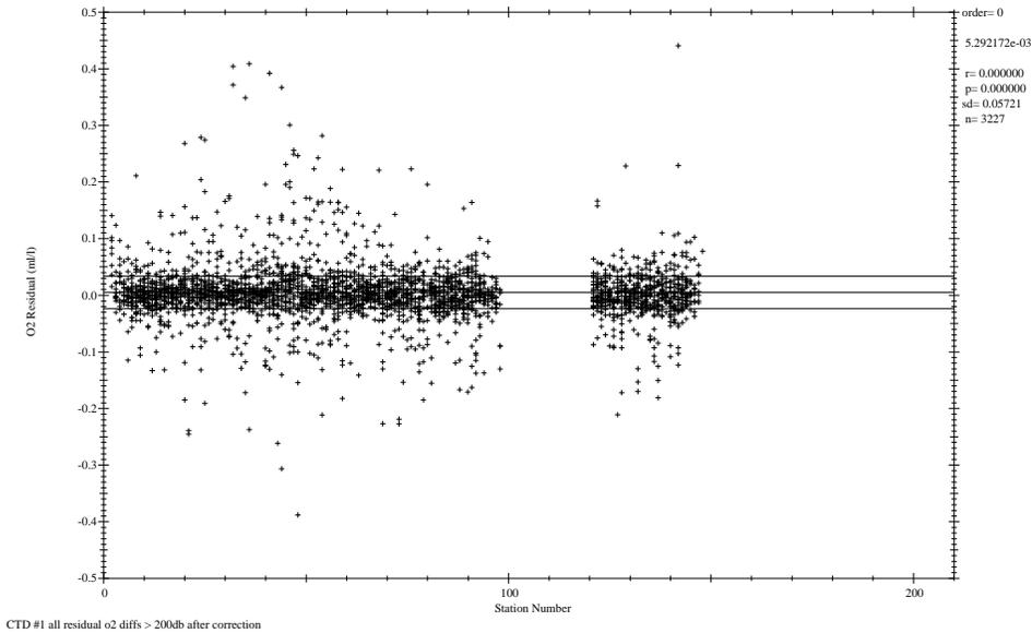
Figure 1.6.6  $O_2$  residual differences vs station # (after correction).
