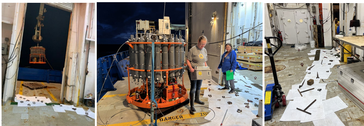
Figure 1.10. Rosette recovery on Station #13. Oil absorbent pads are on the floor due to slippery deck conditions resulting from the hydraulic fluid leakage at Station #11.
