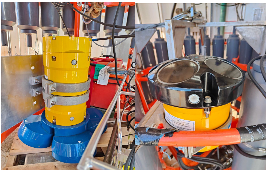
Figure 5.2. (left) Down-facing LADCP mounted behind the CTD package central on the rosette. (right) Up-facing LADCP mounted in place of Niskin bottles 11, 12 on the rosette frame.
