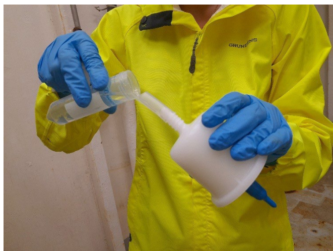
Figure 12.2. Pouring preservation solution into the capsule filter
