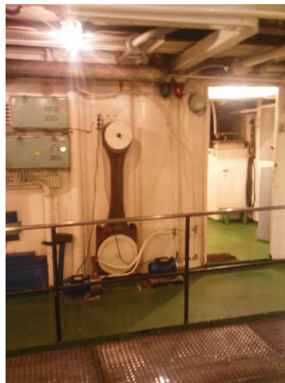
Picture 2.1.1.2 Impeller pumps, Kingston in background.
