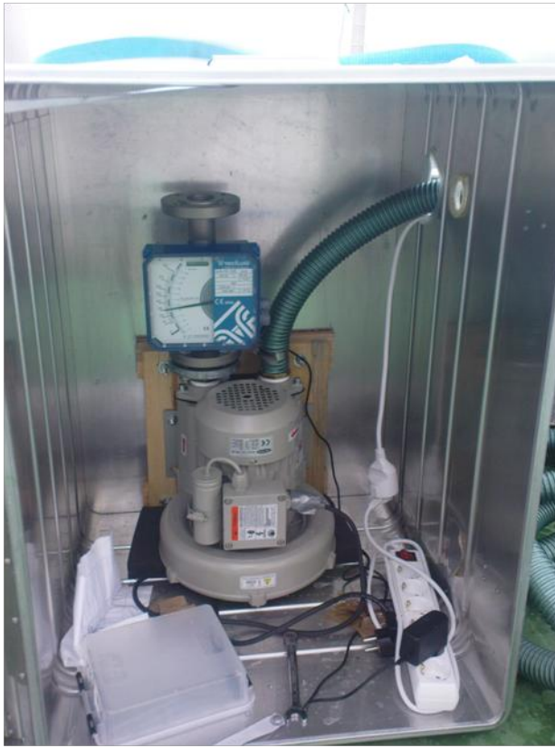
Picture 2.7.1 Pump and flow meter inside box.
