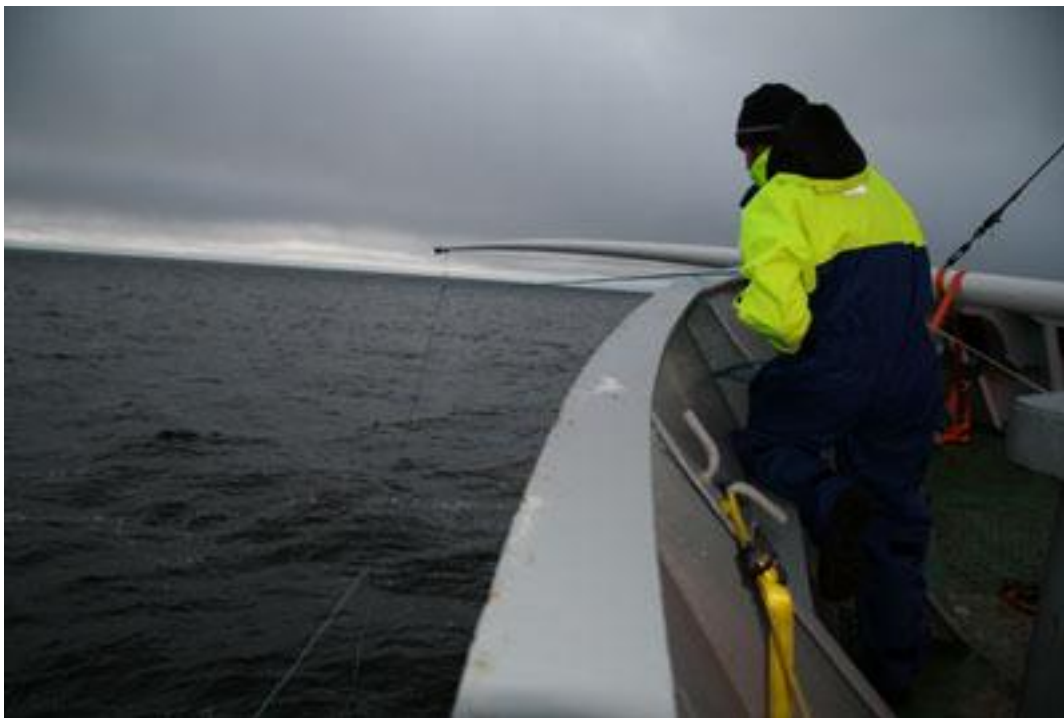
Fig. 2. Flagpole system mounted in the bow of YS for trace metal clean sampling of surface seawater (Photo Jorien Vonk)
