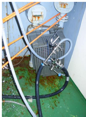
Picture 2.1.1.4 T-piece splitter.
