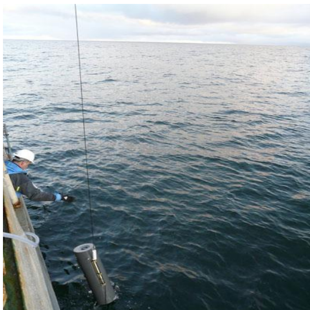
Fig. 1. 60L Go-Flo on Kevlar line with Teflon messenger (Photo Jorien Vonk)
