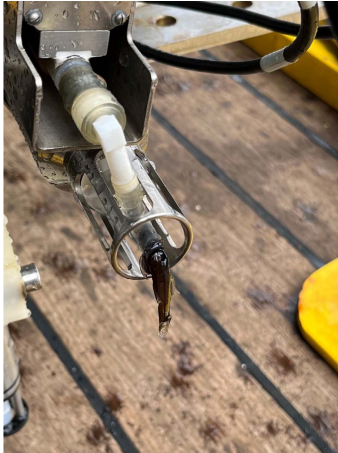
Figure 6.1 Fish blocking primary SBE 3P inlet.
