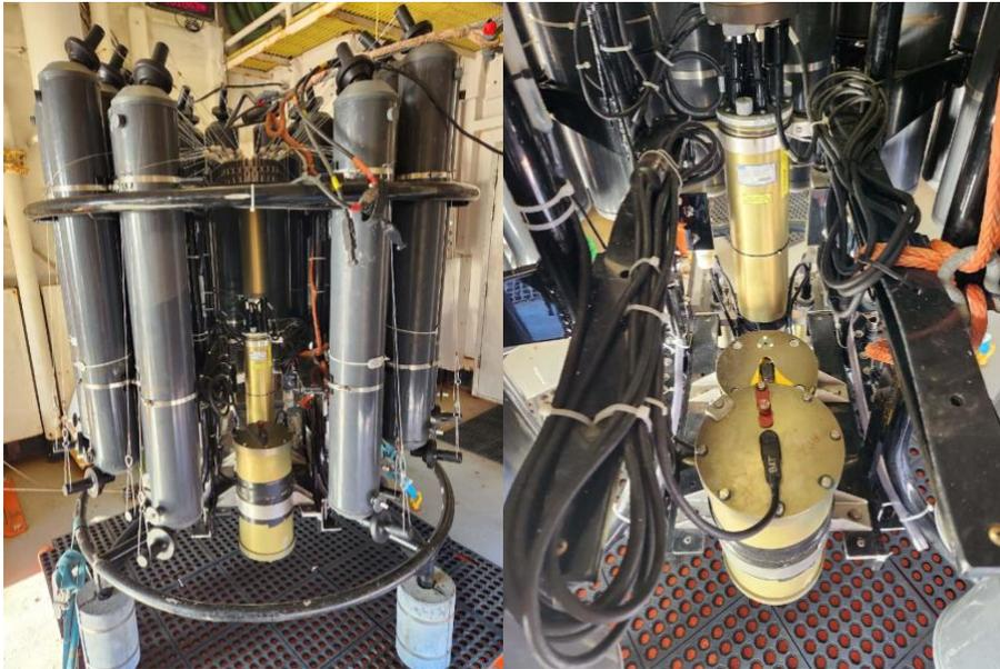
*Figure 6. Complete LADCP package setup for Part II of A16N Leg 1. The left image shows the entire package, while the right highlights the position of the downlooker.*
