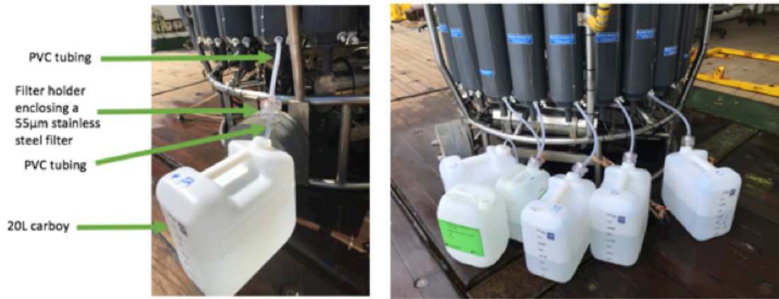
Figure 18.3: CTD sampling for microplastics via a 55 \mu m filter
