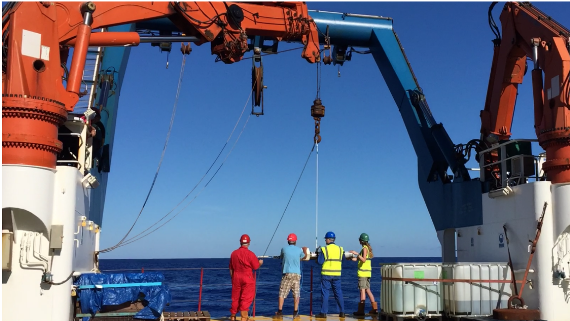
Figure 19.1: Deployment of Argo float of type NKE Provor using a small crane.
