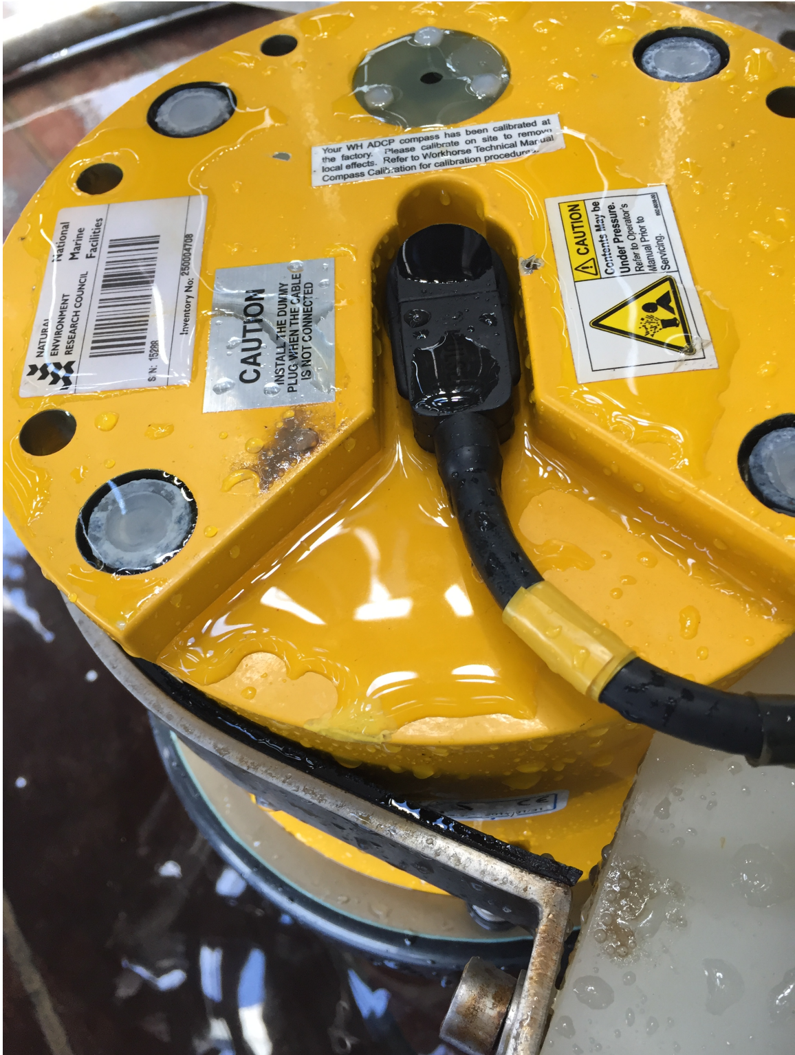
Figure 1.3: Downward-looking LADCP and mounting bracket viewed from above
