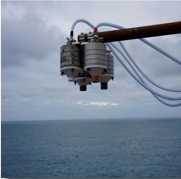
Fig. 3.7.1: Four filter pack systems collecting samples of NH 3 and NH 4 +
