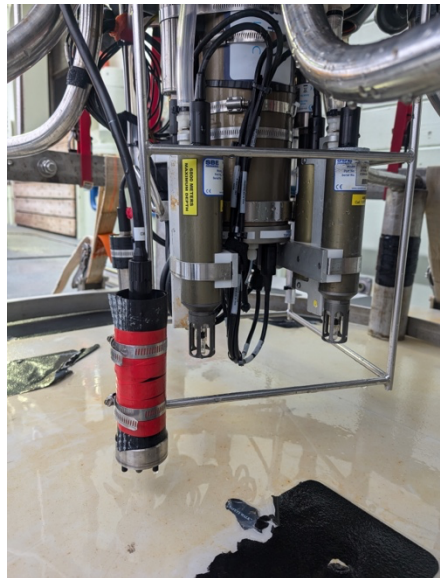
Figure 1: Mount location of the Rinko optode sensor
