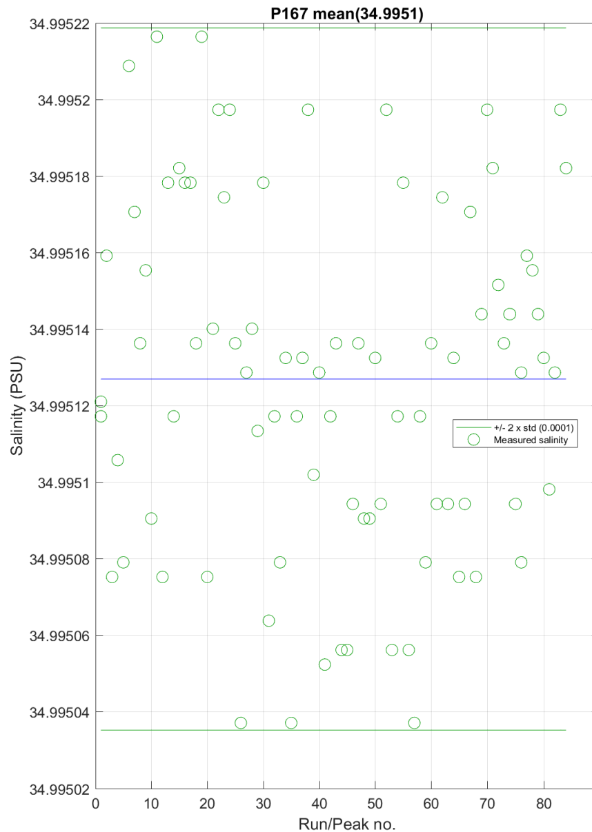
Figure 4. Measured OSIL standard for each salinity run and average value (P167 mean) across IN2024_V01.
