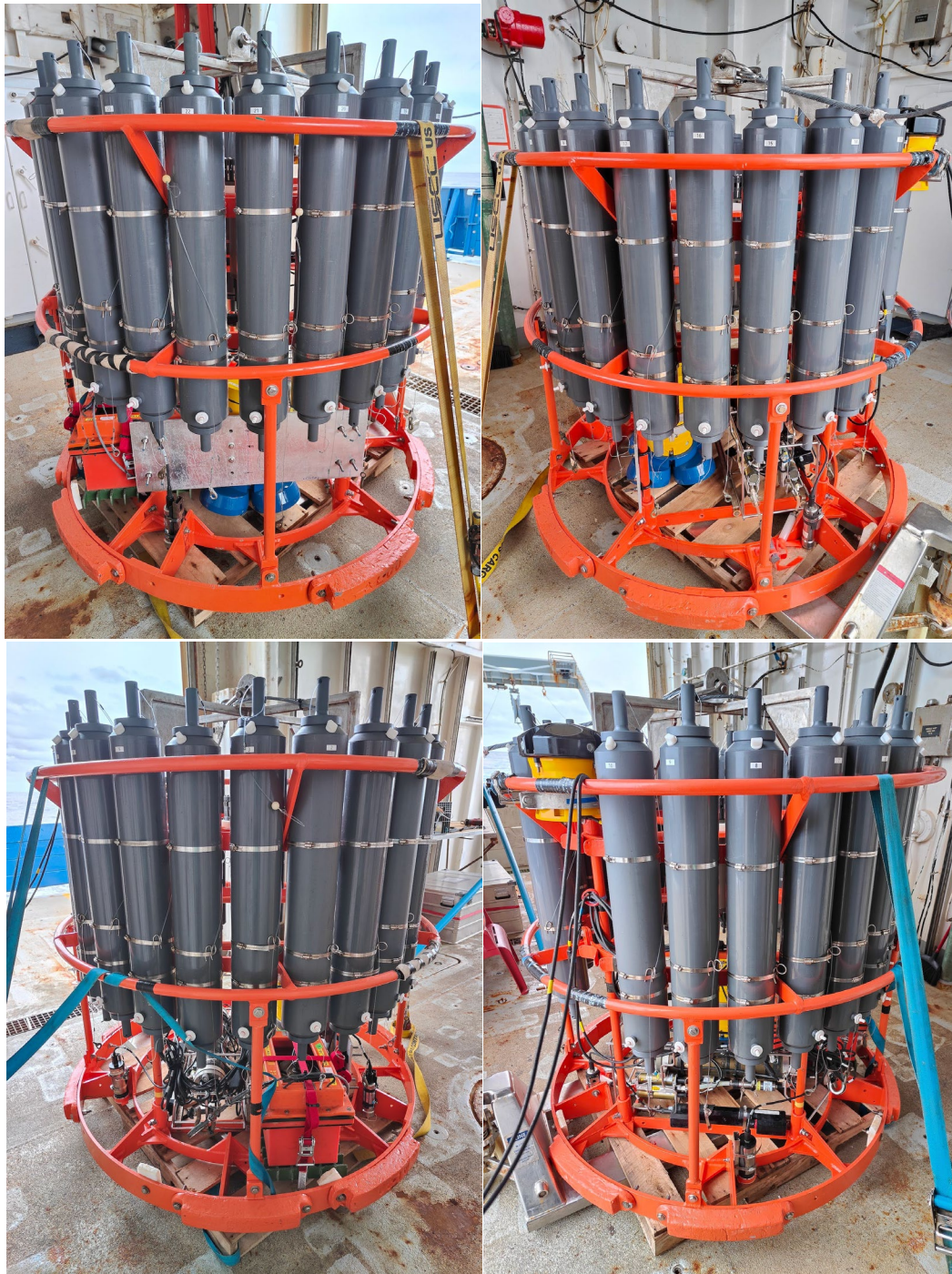
Figure 5.1. Photos of the CTD and rosette, showing the package sensor setup from all sides.
