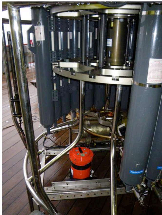
Figure 2.1. The BAS CTD frame and equipment, pictured with some of the Niskin bottles removed. The red instrument is the Bangor LADCP, which replaced the NOCS LADCP for the final two CTD stations (31 and 32).
