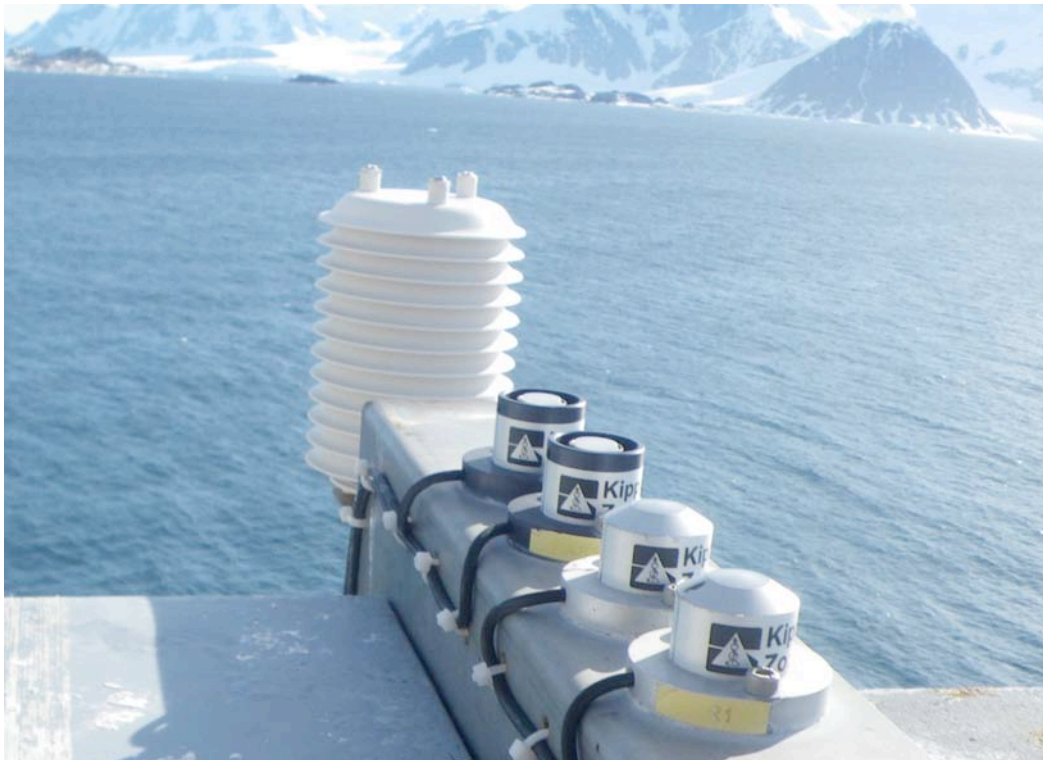
Figure 6.4 The radiation sensors located on the bird table of the foremast platform.
