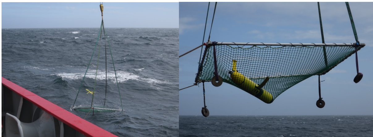
Figure 10: Recovery of a Slocum glider using the net.
