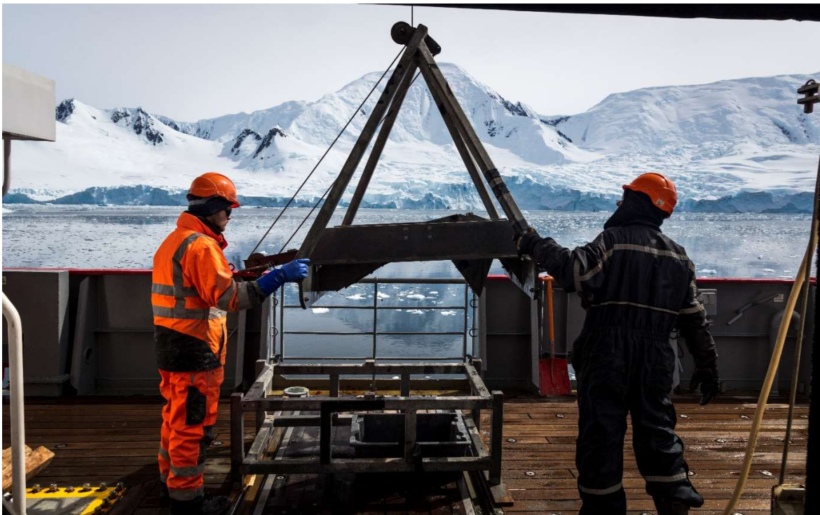
Figure 6.7.1: The Hamon grab is lifted from its stand and hoisted over board. The bucket for collecting the sample can be observed within the grab stand frame. Notice that the swivel mechanism of the grab is in horizontal position (prior to triggering) with the spade bucket on the right side of the grab.
