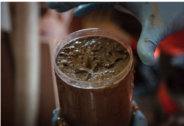
Fig. 6.10.3: Extruding multi-core tube using 1 cm thick Perspex ring to guide sub-sampling.
