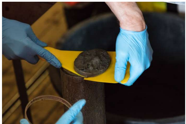
Fig. 6.10.4: Sub-sampling multi-core tube using plastic slicers. cm thick Perspex ring to guide sub-sampling.
