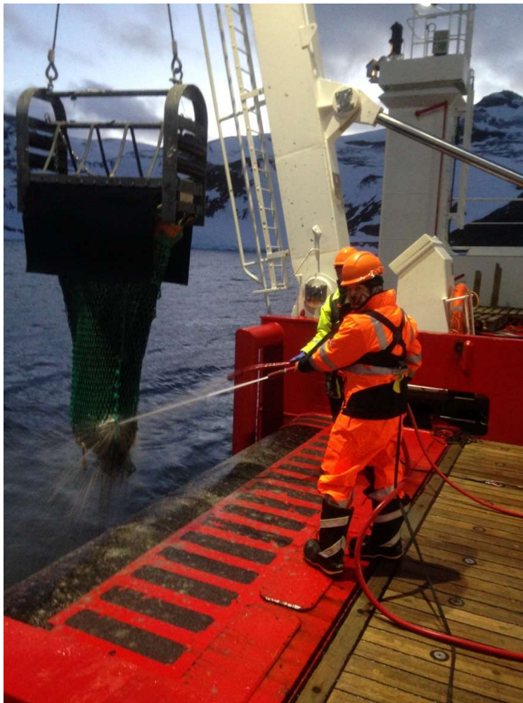
Figure 6.9.1 miniAGT being recovered. Fire hoses were used to wash out mud before landing the trawl on the deck.
