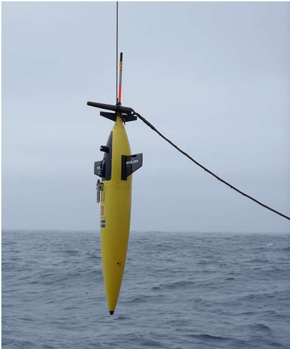
Figure 10.1.4: The Seaglider on deployment. One line feeds up to the aft crane, with an eye looping around the base of the rudder. The eye is held in place by the wooden toggle, which is removed for deployment.
