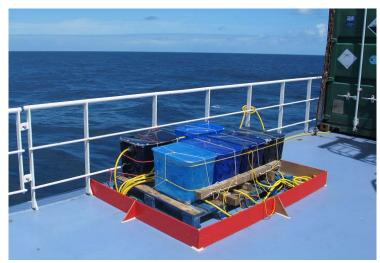
Figure 1. Incubators for the 6 different depths with adjusted light lifters (54%, 25%, 13%, 3%, 1%, 0.2%) as setup during the Geovide cruise
