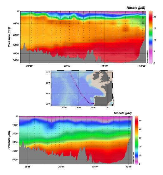
Nitrate measured on the TMR-stock will be used for the interpretation of the trace metal profiles, but also served to check for potential leakage on the Go-Flo bottles. As an example below, at station#21, at 2800 m the Go-Flo#5 was leaking and the measurement will not be considered in the data set.
