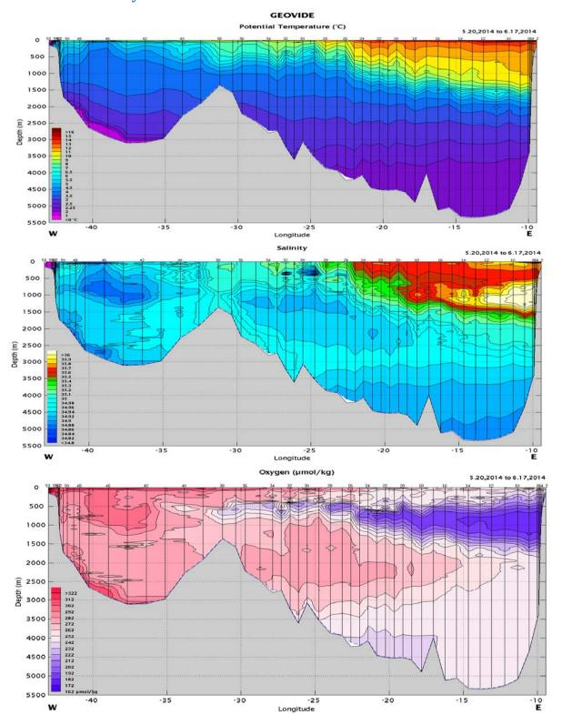
**Figure 4**: Sections of temperature (top, in °C), salinity (middle) and dissolved oxygen (bottom, in µmol/kg) between Greenland (left) and Portugal (right), as a function of longitude. Those sections were done with the pre-calibrated data of the first downcast of each station (hydrological rosette).
