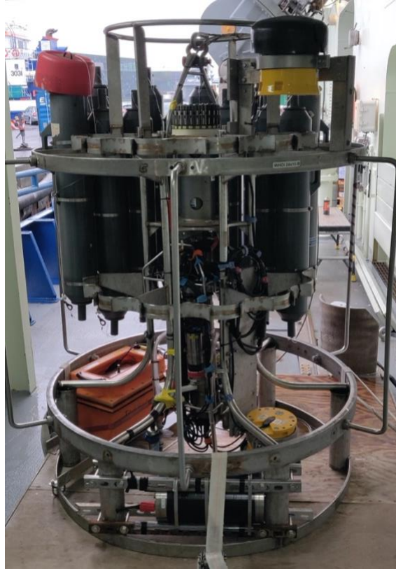
Figure 6 Niskin rosette with additional bottles removed to view CTD plumbing and carousel (Photo F. Straneo, SIO).
