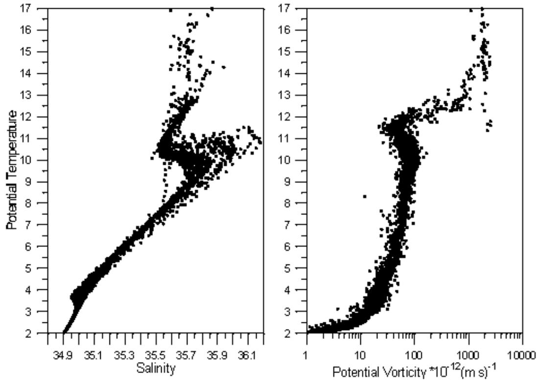
**Figure 6.** Diagrams of salinity and potential vorticity versus potential temperature. The data are from all CTD casts, sub-sampled every 50 dbar.
