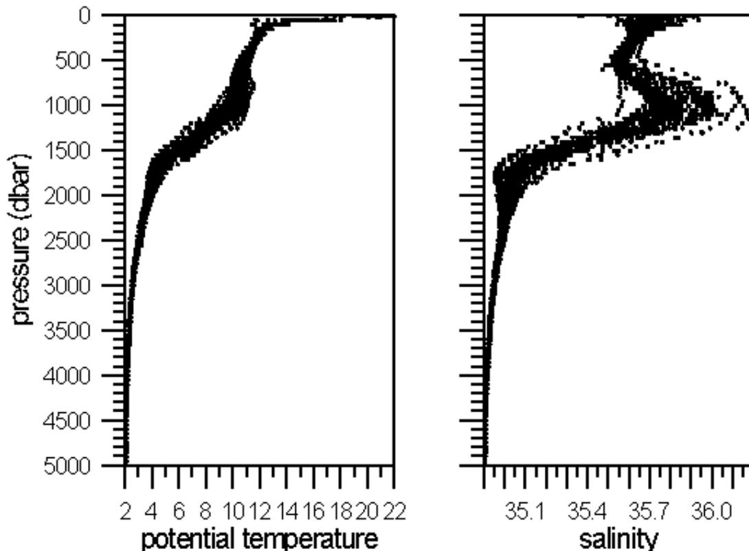
**Figure 5.** Vertical distribution of potential temperature and salinity from all CTD casts, sub-sampled every 50 dbar.
