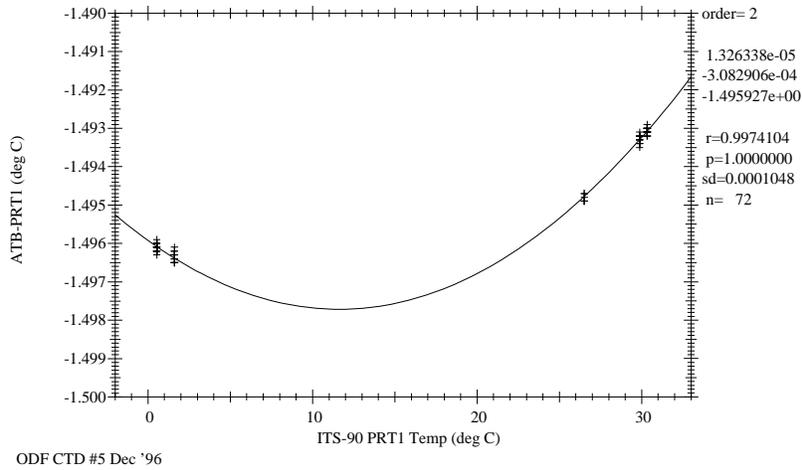
**Figure 7.3** Primary PRT Temperature Calibration for ODF CTD #5, December 1996.
