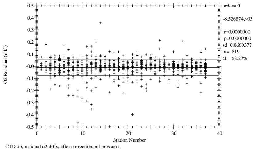
Figure 8.4.0 ICM3  $O_2$  residual differences vs station # (after correction).
