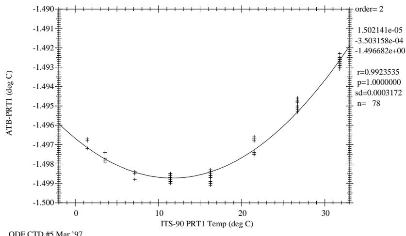
**Figure 7.5** Primary PRT Temperature Calibration for ODF CTD #5, March 1997.
