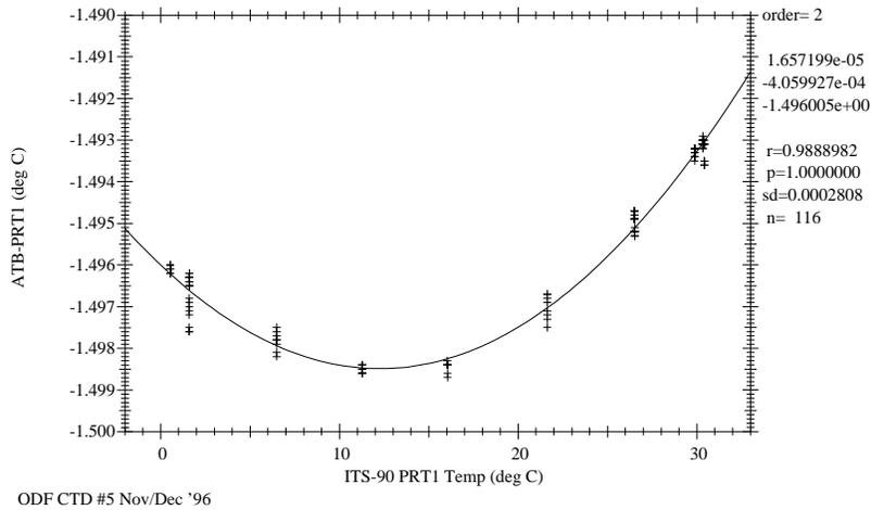
**Figure 7.4** Primary PRT Temperature Calibration for ODF CTD #5, Combined Nov.+Dec. 1996.
