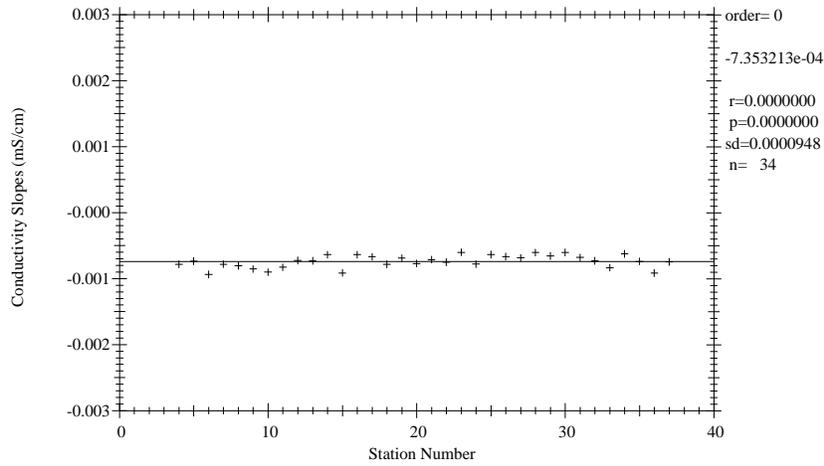
**Figure 8.3.0** ICM3 CTD #5 preliminary conductivity slopes by station number.
