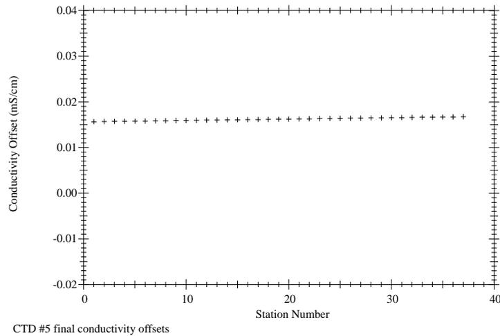
**Figure 8.3.3** ICM3 CTD #5 conductivity offsets by station number.
