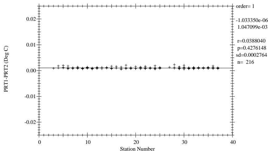
**Figure 8.2.0** Shipboard comparison of CTD #5 primary/secondary PRT channels, pressure>2000db.
