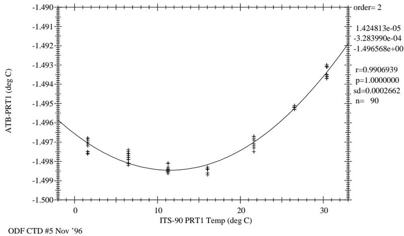
**Figure 7.2** Primary PRT Temperature Calibration for ODF CTD #5, November 1996.
