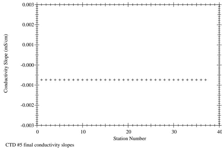
**Figure 8.3.2** ICM3 CTD #5 conductivity slope corrections by station number.
