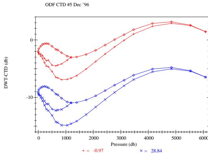
Figure 7.0 Pressure calibration for ODF CTD #5, December 1996.
