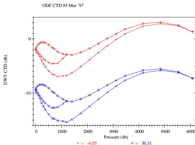
Figure 7.1 Pressure calibration for ODF CTD #5, March 1997.
