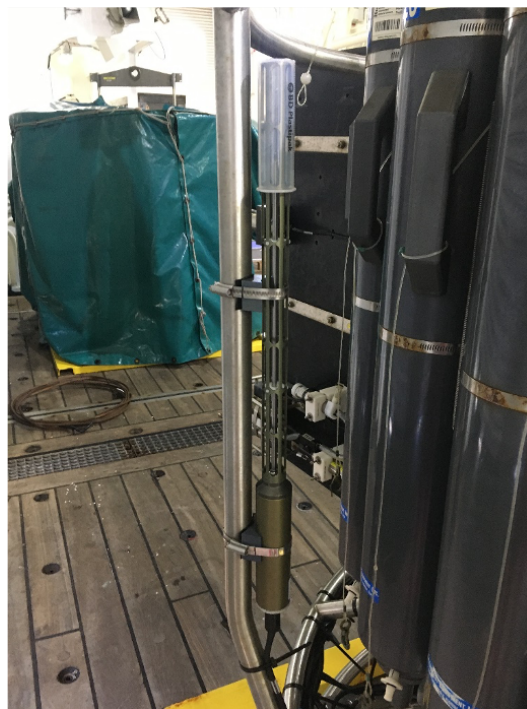
Seabird SBE 35 DOST Mounting Location Overview
