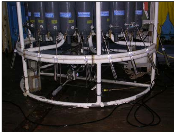
Figure 3.2a: CFC sampling containers attached to the carousel water sampler (Foto by U. Stöber).
