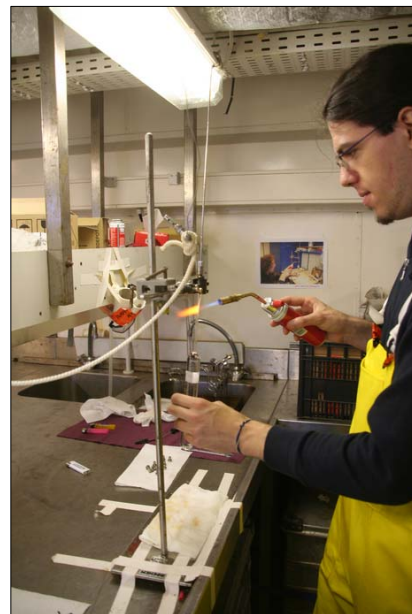
Figure 3.2b: Sealing CFC sample ampoules (Foto by D. Kieke).
