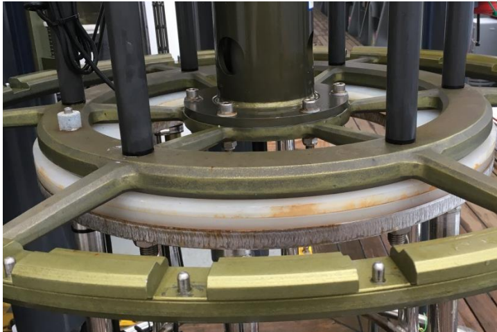
Figure 16:- Installation of additional CTD isolation washer
