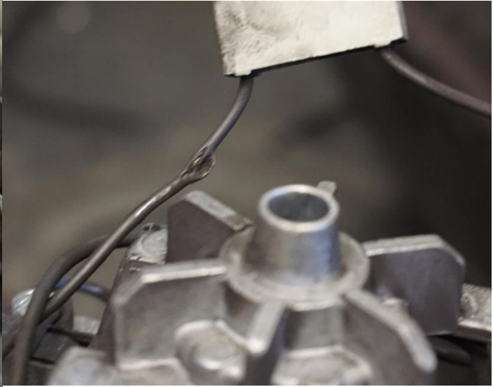
Figure 24:- UEA damaged capacitor wire
