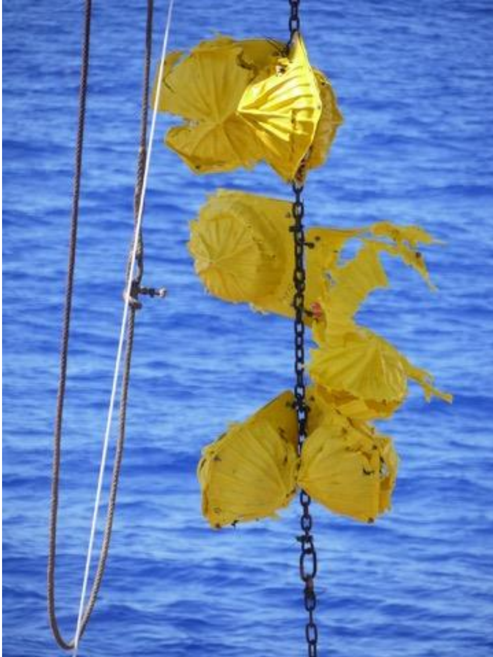
Figure 4: Imploded buoyancy spheres.
