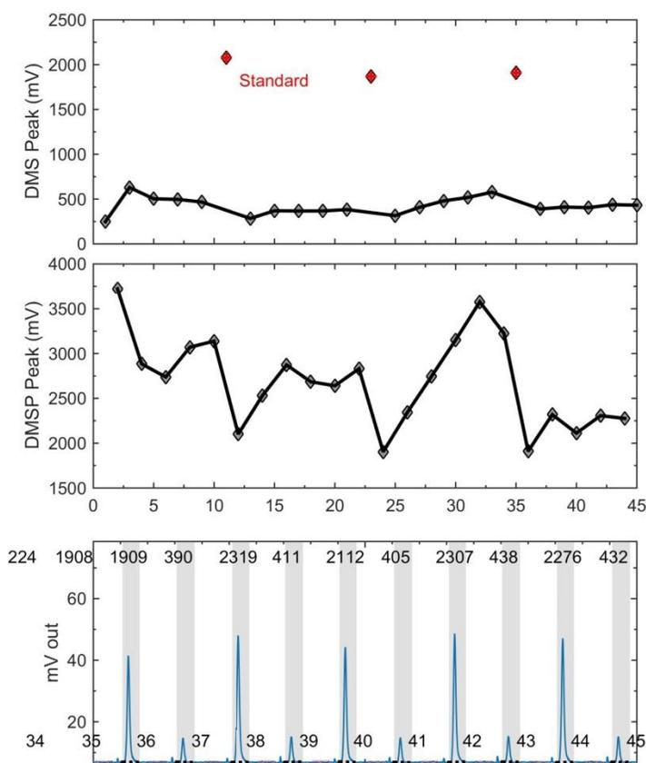
**Fig.1.** Sample data obtained for underway analysis of DMSP and DMS using the OSSCAR system. The bottom panel shows peaks eluting from the GC column. Numbers at the top are the peak integrals computed in real-time using a matlab script. The top two panels show the peak areas for DMS and DMSP over the sequence of a 45 sample run.
