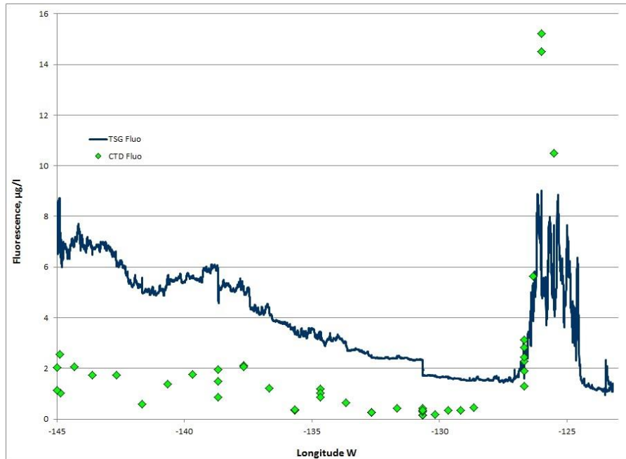
Figure A: Fluorescence from the Thermosalinograph and from the CTD along Line P, outbound leg.
