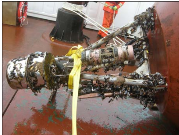
Before (left) and after (right) deployment at Ocean Station Papa. The sensors are covered in copper foil to reduce fouling. The SAMI-pH sensor is the upper instrument in both pictures; the SeaBird CTD package is the lower set of instruments.
