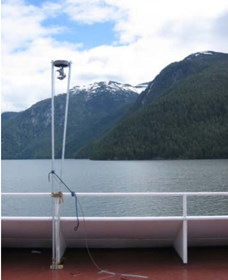
Figure 2. Gimble PAR sensor mounted on deck above bridge.
