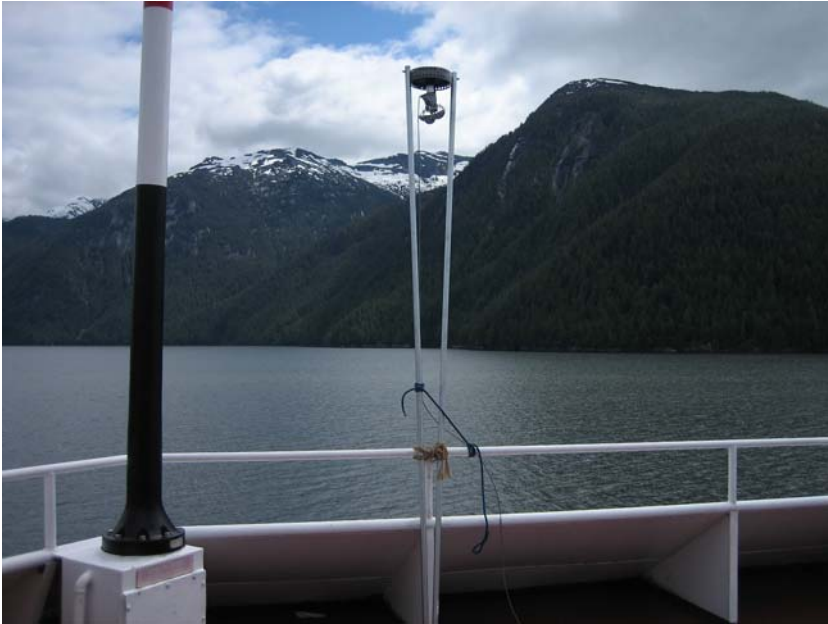
Figure 2. Biospherical Instruments PAR sensor on gimble mast above Tully heli deck.
