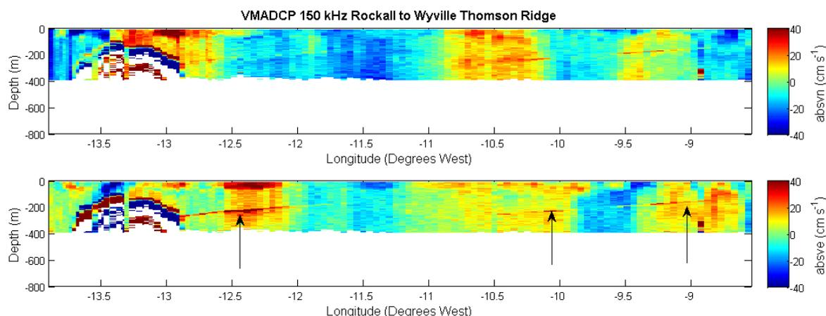
Figure 3.3: Example of 4 km averaged 150 kHz VM-ADCP data from Rockall to the Wyville Thomson Ridge. Positive velocities indicate northward currents (top plot) and eastward currents (bottom plot), negative velocities indicate southward currents (top plot) and westward currents (bottom plot). Arrows indicate the position of sloping lines in 150 kHz data. The velocity scale has been limited to  $40 \text{ cm s}^{-1}$  to present maximum detail within the data.
