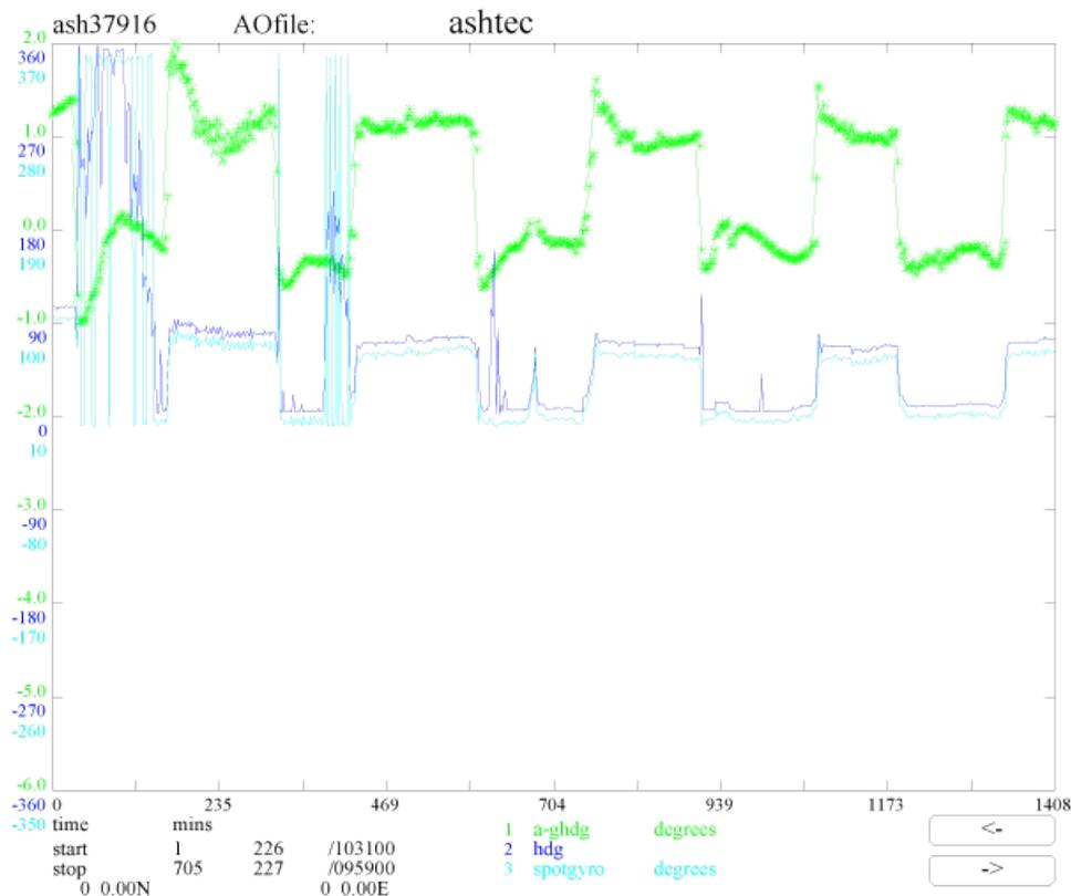
**Figure 3.1. Example of the onscreen output of daily navigation hdg data generated by gyro (light blue line), ashtech ADU5 (dark blue line) and the difference between them (green line).**
