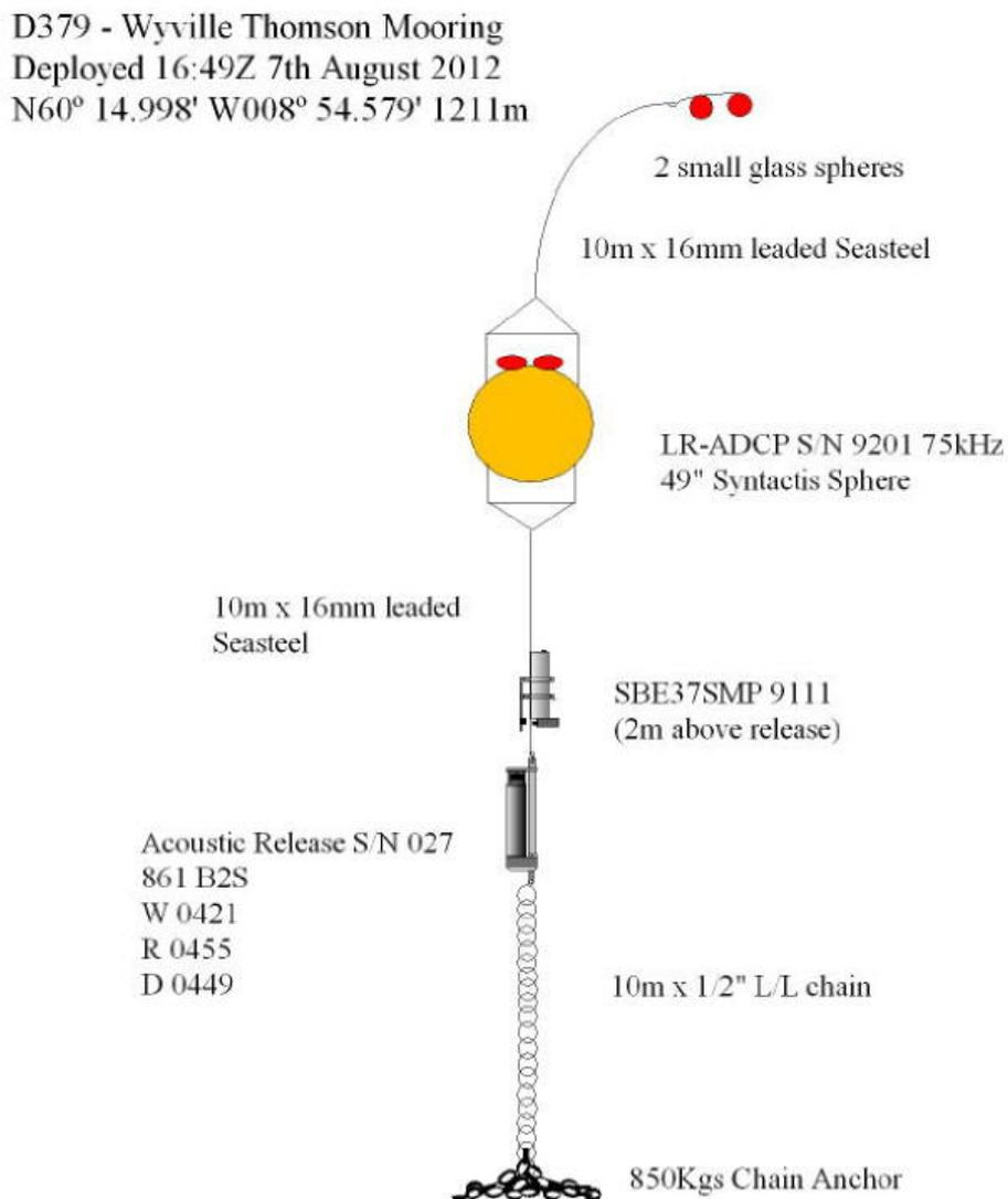
Figure 11.2 - Deployed WTR Mooring
