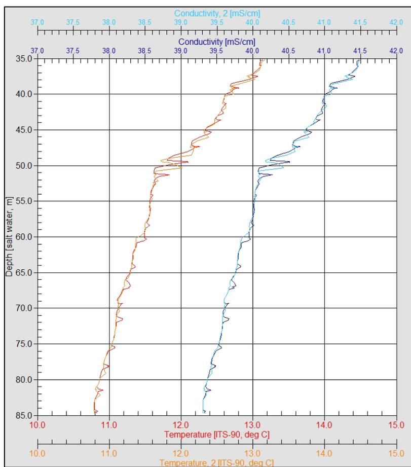
**Figure 2.4: Typical spiking observed on CT sensors in the thermocline area (example from cast 25)**
