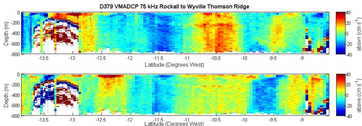
Figure 3.4: Example of 4 km averaged 75 kHz VM-ADCP data from Rockall to the Wyville Thomson Ridge. Positive velocities indicate northward currents (top plot) and eastward currents (bottom plot), negative velocities indicate southward currents (top plot) and westward currents (bottom plot). The velocity scale has been limited to  $40 \text{ cm s}^{-1}$  to present maximum detail within the data.
