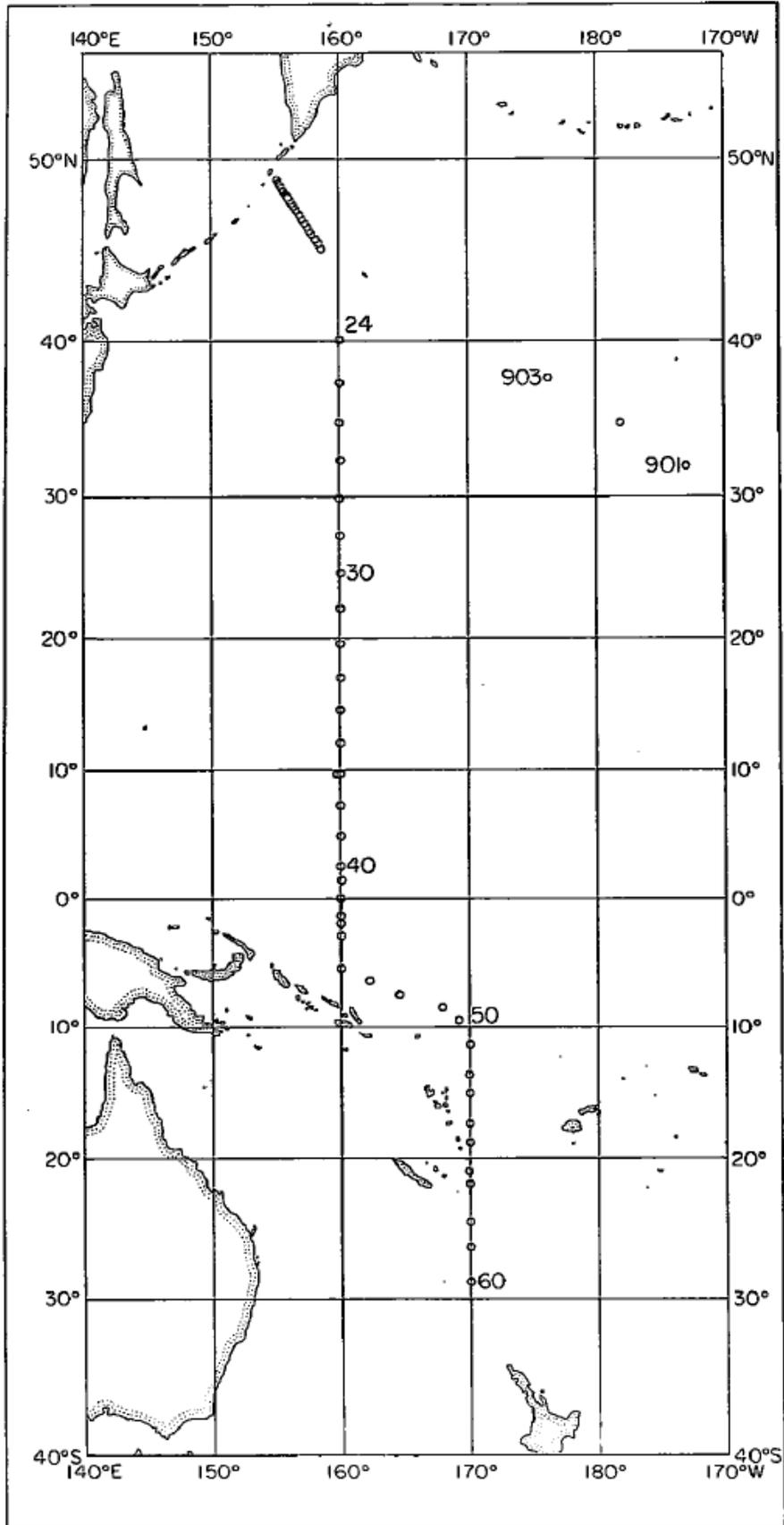
The CTD/hydrographic work consisted of three parts: 3 test stations, 23 closely-spaced, deep stations in the northwest Pacific across the Kuril-Kamchatka Trench, and 37 shallow stations along 160°E and 170°E between 40°N and 28°S.
