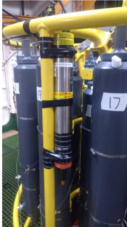
Fig. 18.1: Chipod pressure case attached on the rosette
