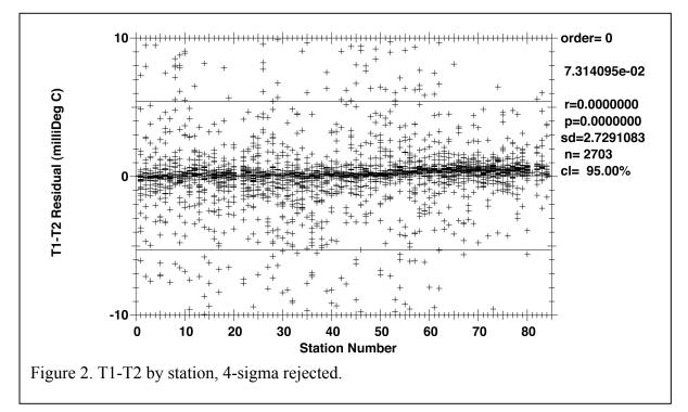
The 95% confidence limit for the mean of the differences is  $\pm -0.0073$ °C. The variance is relatively high in spite of the small spatial separation of the sensors ( $\leq 0.5$  meters) because of package wake effects.
