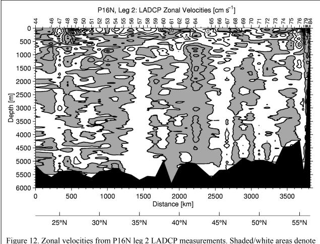
westward/eastward flow. Contour interval is 5 cm s<sup>-1</sup>.
