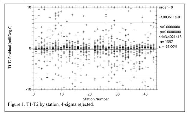
The 95% confidence limit for the mean of the differences is  $\pm -0.0068$ °C. The variance is relatively high in spite of the small spatial separation of the sensors (< 0.5 meters) because of package wake effects.
