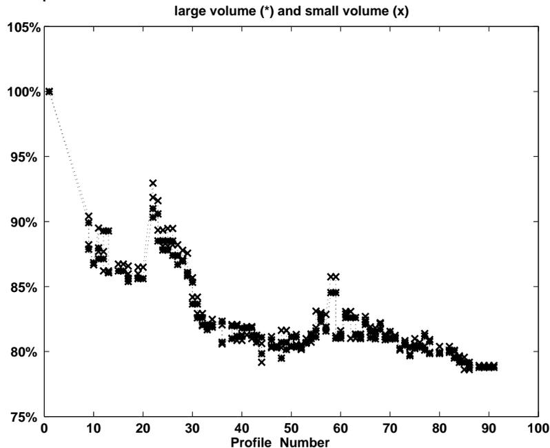
Figure 2: The temporal evolution of the ECD-efficiency during the cruise for the 0.5 mL volume (small) and the 2 mL volume (large).
