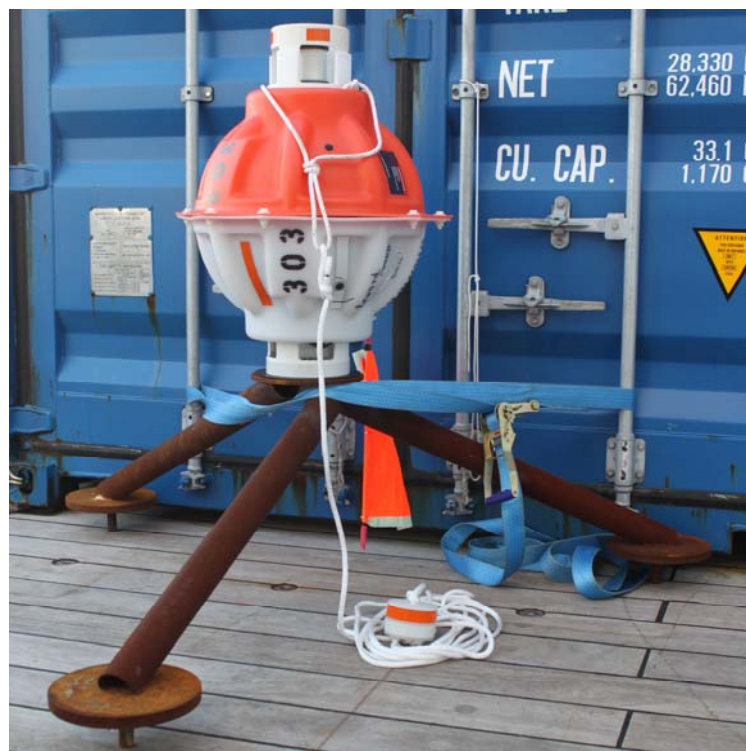
Fig. 5.13 Inverted echo-sounder equipped with pressure sensor (PIES, s/n 303) which is fixed on a tripod that serves as a bottom weight. Attached are a flag and a pick-up line that will facilitate retrieval and recovery at the end of its mission. Photo by A. Roessler.
