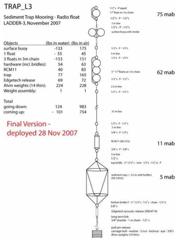
**Figure 6.1.** Diagram of TrapL3 mooring near Sketchy vent, for recovery in Fall 2008
