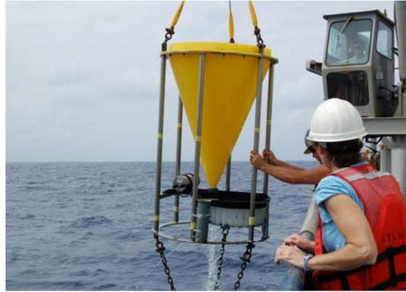
**Figure 2.2.** Recovery of sediment trap on LADDER3. Collected material is visible in white cups below cone (photo by S. Bayer)
