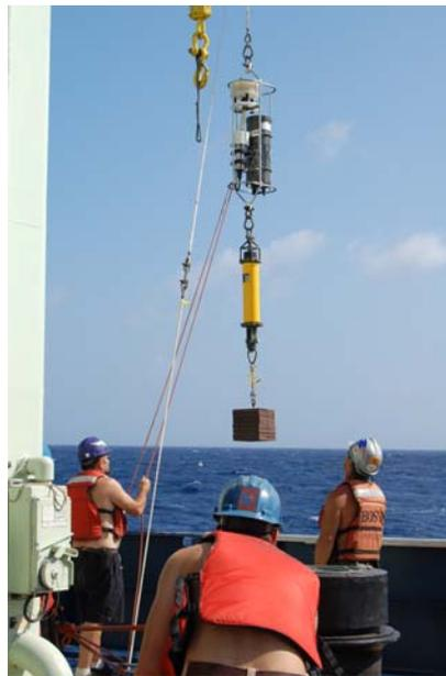
**Figure 2.1.** Deployment of McLane plankton pump, using anchor-first method of lowering on wire (photo by S. Mills)
