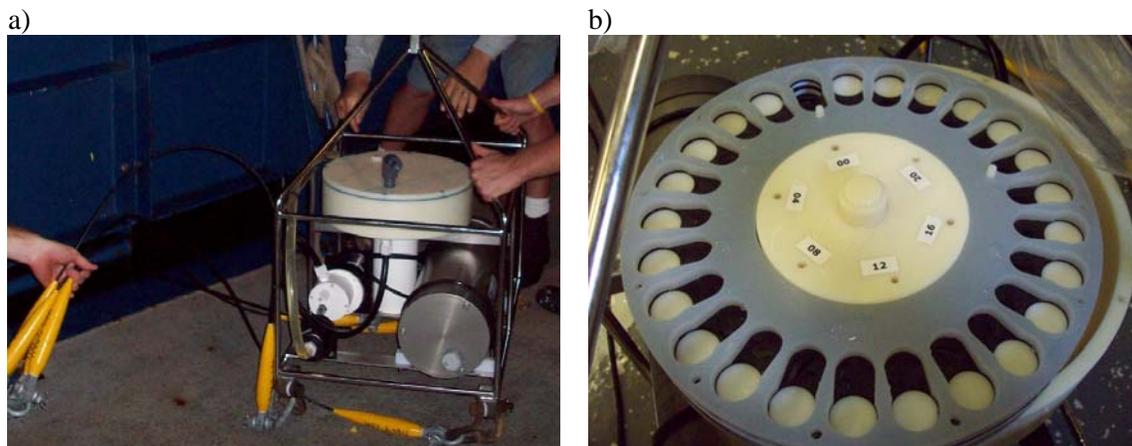
**Figure 4.6.** The a) SUPR sampler contains a b) rotating filter rosette driven by a stepper motor. The water inlet and outlets, and future optical sensor and dosing ports, are stationary. Fused silica windows will be added to the current filter rosette to complete the optical design.
