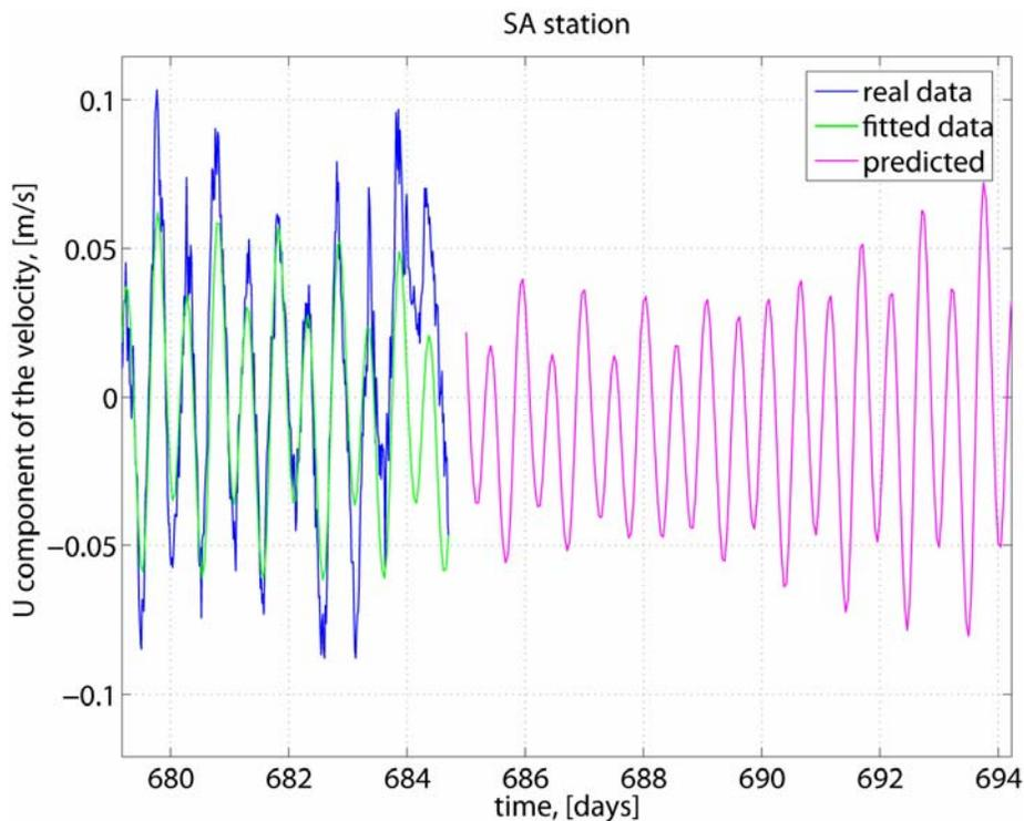
**Figure 3.2.** Tidal fit and prediction based on a current meter from the SA mooring. The data extracted from the CM are shown in blue, the corresponding fit in green, and the resulting prediction in magenta.
