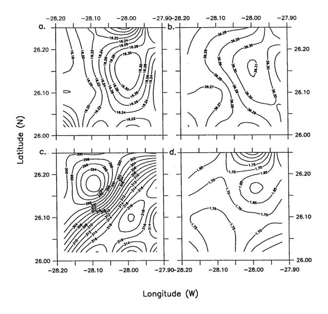
**Figure 14:** Contour plots of potential temperature (a) salinity (b) pressure (c) and density ratio (d) on the  $\alpha_{300}$  = 28.00 surface for the small scale survey
