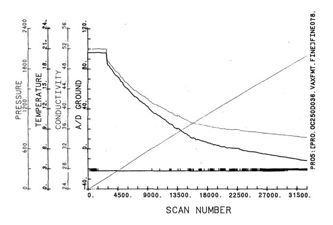
**Figure 5a:** Plot of Pressure, Temperature, Conductivity, and A/D ground versus scan number for dive 78.
