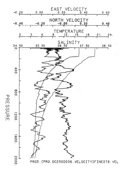
**Figure 6:** Plot of computed velocity (east and north components), temperature and salinity versus pressure for dive 78.
