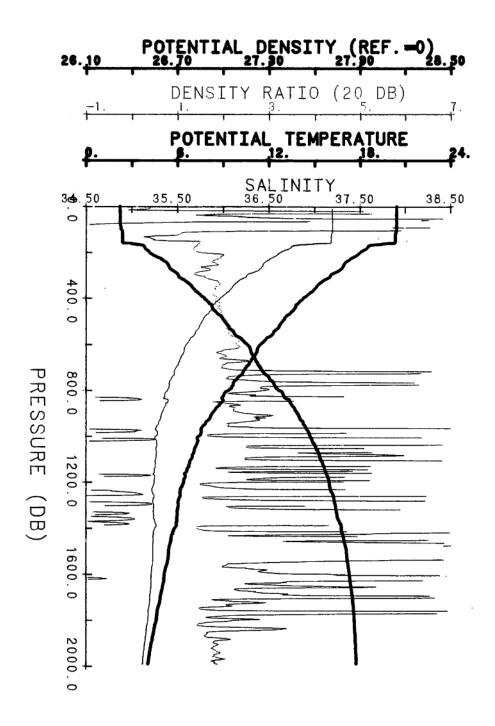
**Figure 8:** Profiles of potential temperature, salinity, potential density and density ratio versus pressure (computed from finescale data variables) are shown for dive 78.
