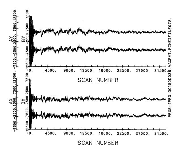
*Figure 5b:* Plots of accelerometer data for dive 78. The upper plot shows the y component of the two accelerometers and the lower plot shows the x components of the two accelerometers.
