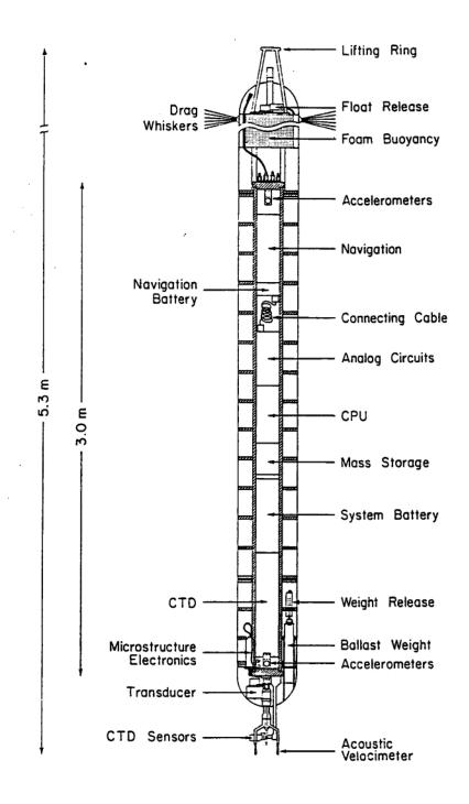
Figure 4: Schematic of the High Resolution Profiler (HRP)
