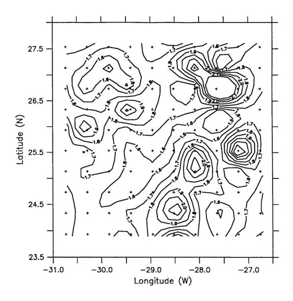
Figure 12: Contour plot showing the density ratio field at 300 db for the large scale survey.
