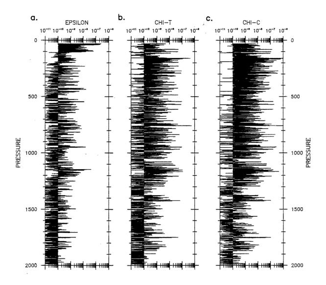
**Figure 7:** Plots of energy dissipation rate, epsilon (a), dissipation rate of thermal variance from micro- temperature (b), micro-conductivity (c) sensors for dive 78.
