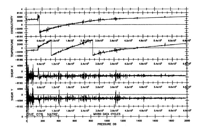
**Figure 5d:** Example of a microstructure data quality control plot using dive 78. Micro-temperature, micro-conductivity, shear x and shear y are plotted against scan number.
